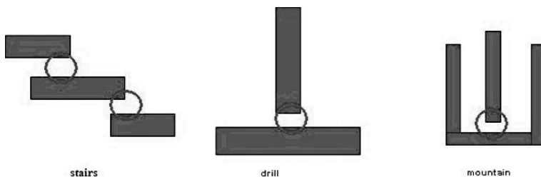
Figure 3.24. Three Known Problem Patterns from a 65nm LRC Library
