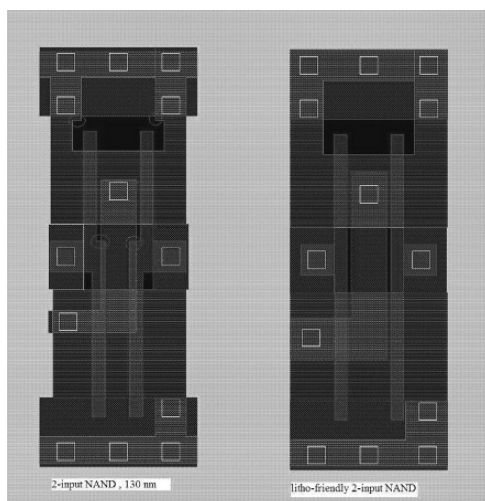
Figure 3.29. Old Style “Compact” Layout vs Litho-friendly Cell Layout
