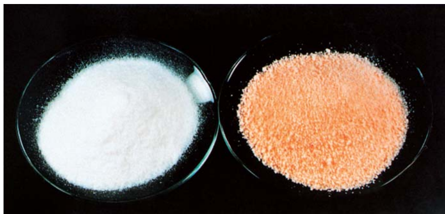
Fig. 44. The influence of different methods of wet granulation on the colour stability of an ascorbic acid granulate with povidone K 30 (after 6 months at room temperature) Left: Fluidized bed granulate. Right: Diosna Mixer granulate
