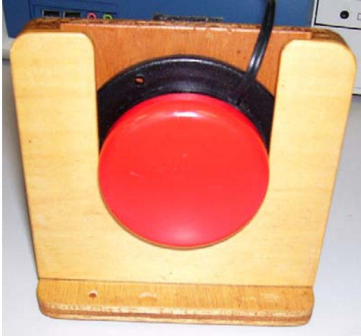
Figure 3. Vertically Mounted Large (13cm Diameter) Jelly Bean Switch. © 2010 Helen J. Farrell. Used with permission.
