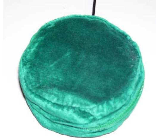
Figure 4. Soft Pad Switch. © 2010 Helen J. Farrell. Used with permission. See Beukelman & Mirenda, 2005.
