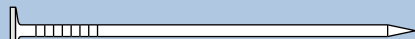
Cement-coated box: coated with resin that melts on driving and acts as adhesive
