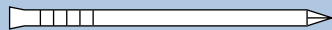
Casing: similar to finish nail but with dulled point for nailing trim without splitting
