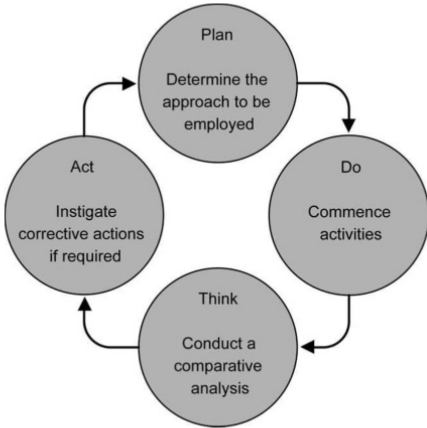
Figure 4.9 Deming's dynamic control loop cycle
