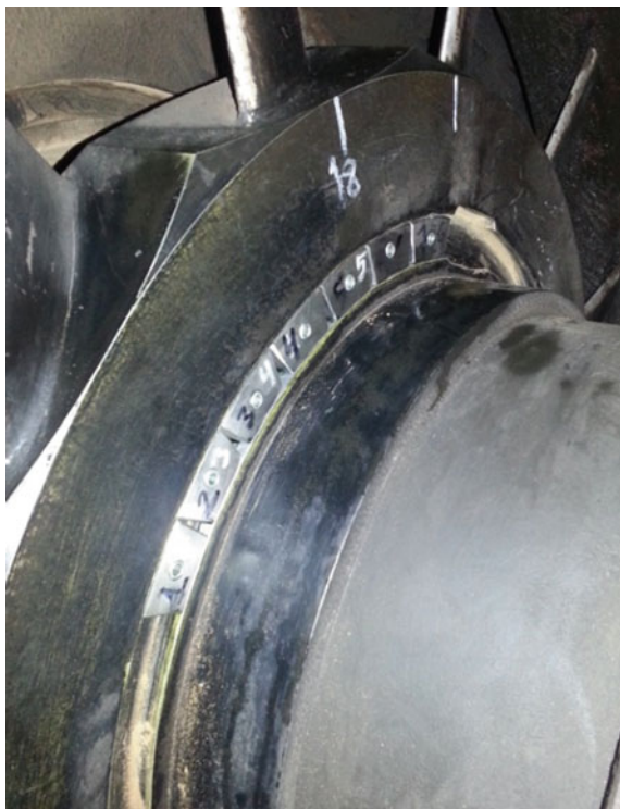
Fig. 5.35 Example of end balance plane weights on a generator rotor
