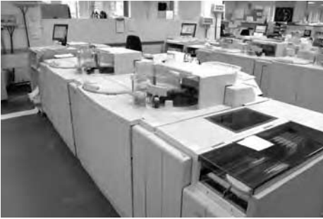
Figure 1.10 A typical automated analyzer in a hospital clinical chemistry laboratory capable of performing most of the major investigations. Courtesy of the Department of Clinical Biochemistry, Manchester Royal Infirmary, UK.
