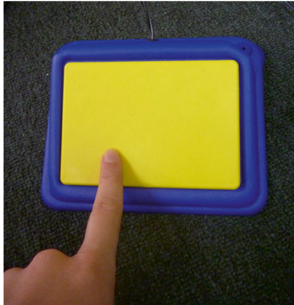
Fig. 2.3 Example of a single-switch AAC device. Photo credit: Jennifer Ninci. Used with permission
