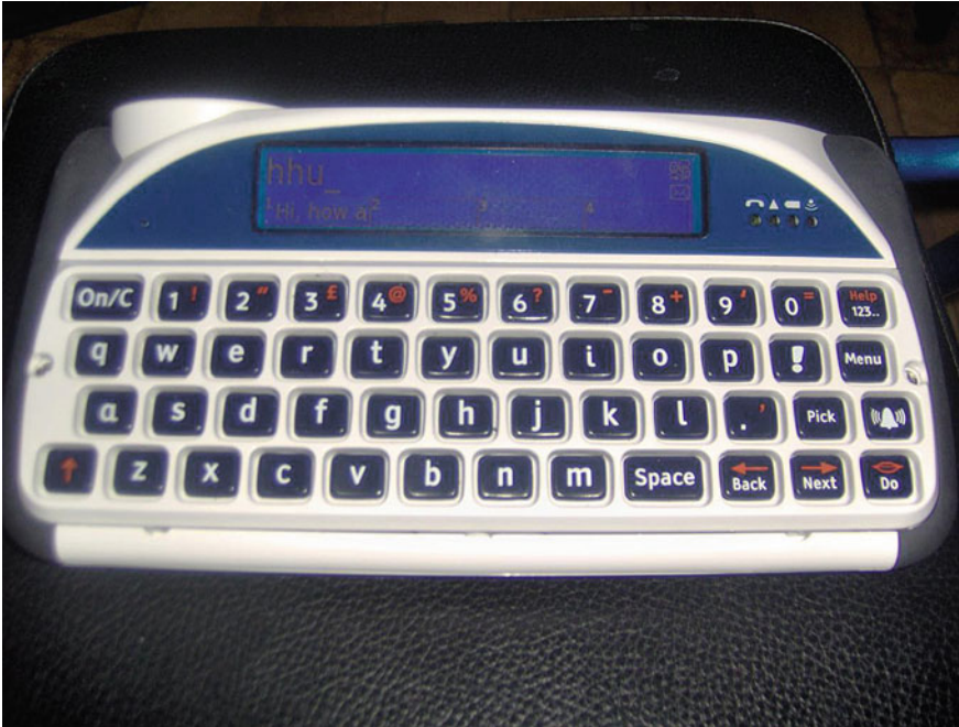
Fig. 4.3 Photograph of a LightWriter. The LightWriter is a text-to-speech SGD manufactured by Toby Churchill Limited in the United Kingdom ( http://www.toby-churchill.com )
