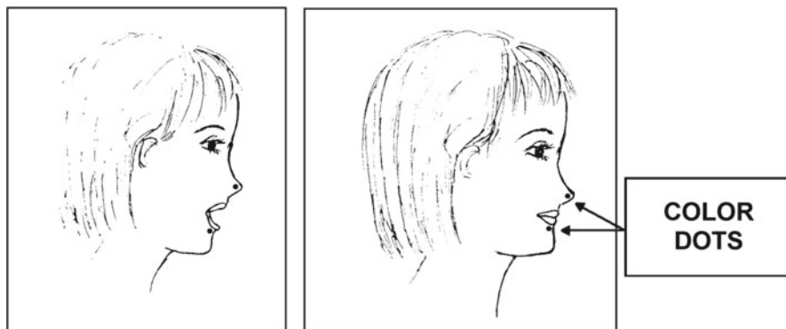
Fig. 2.6 Schematic representation of possible color dots used to detect mouth closing with a camera-based microswitch
