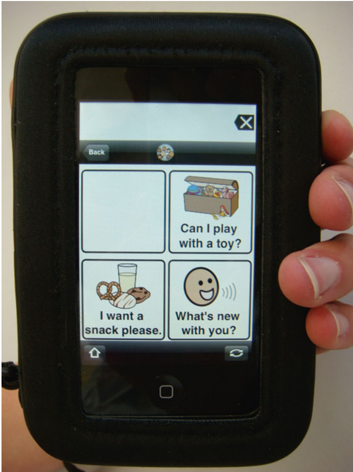
Fig. 3.3 Photograph of an iPod Touch® that has been configured for use as an SGD. The iPod is placed inside an iMainGo® 2 speaker case to improve sound amplification. The visual display shows three graphic symbols for snacks, toys, and social interaction. Lightly tapping each symbol produces corresponding synthesized speech output (e.g., can I play with a toy ) that is preprogrammed using Proloquo2Go™ software
