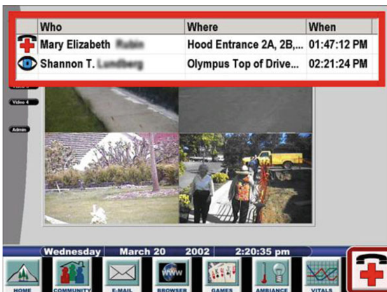
Fig. 12.10 When residents with cognitive impairments approach the edge of the Oatfield Estates campus, their badges signal the automated care system, and a WebCam captures their image and alerts caregivers in case redirection is necessary
