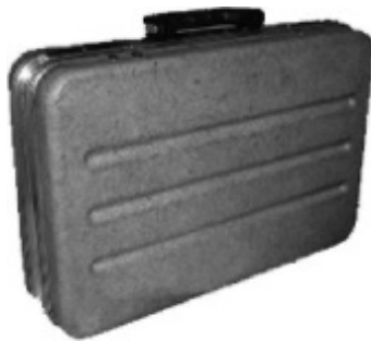
Figure 9.22 Flax fiber composite molded brief case made with flax fiber and polypropylene compression molded non-woven material. Image taken from Ref. [70], copyright © 2006–2018 Stemergy. All rights reserved.
