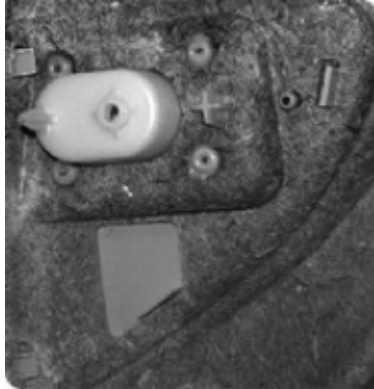
Figure 9.21 Flax fiber–based automotive interior trim part shown with flax fiber composite substrate and plastic inserts for fastening. Image taken from Ref. [70], copyright © 2006–2018 Stemergy. All rights reserved.
