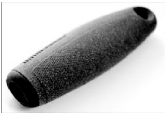
Figure 9.16 Cork produced using injection molding. Reprinted from Ref. [56], with permission from Elsevier.
