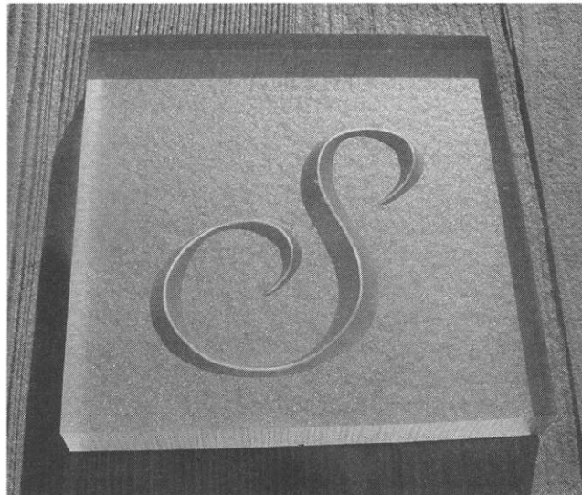
FIGURE A-11 Lettering reverse-engraved into 1/2-in acrylic.
