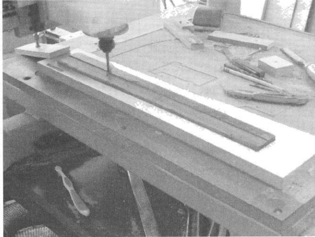
FIGURE A-43 3D routing of a compound radius on the fret board.
