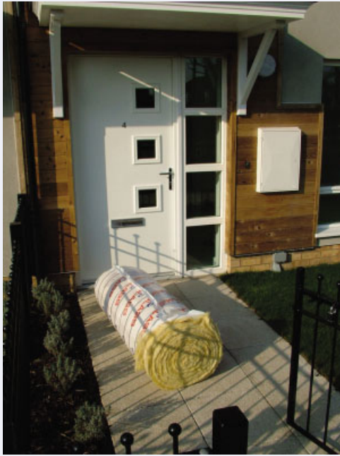
Figure 2.23 Domary Court: fibreglass insulation used in roof
