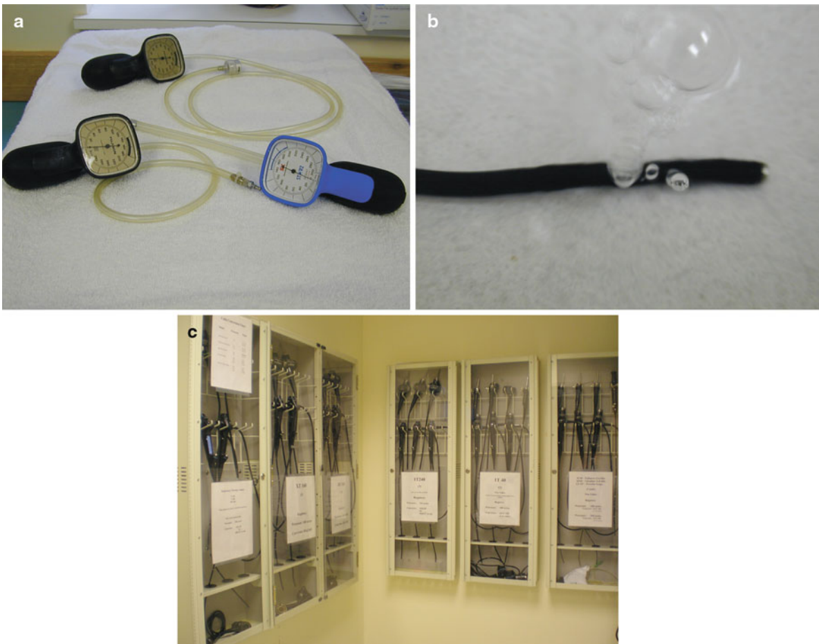
Fig. 3.8 (a) Leak tester. (b) Bronchoscope leak with bubbles after pressurization. (c) Bronchoscopy storage
