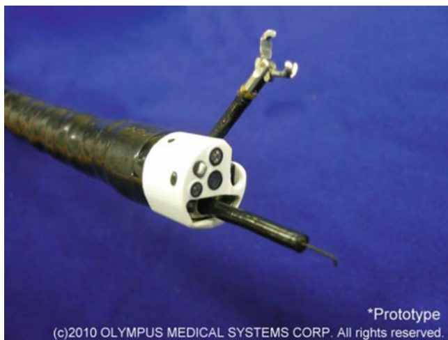
Fig. 69.3 Another NOTES prototype with steerable working channels is shown
