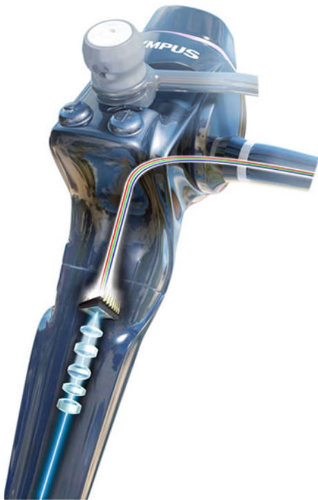
Fig. 2.17 Placement of the CCD inside the control section of a hybrid scope
