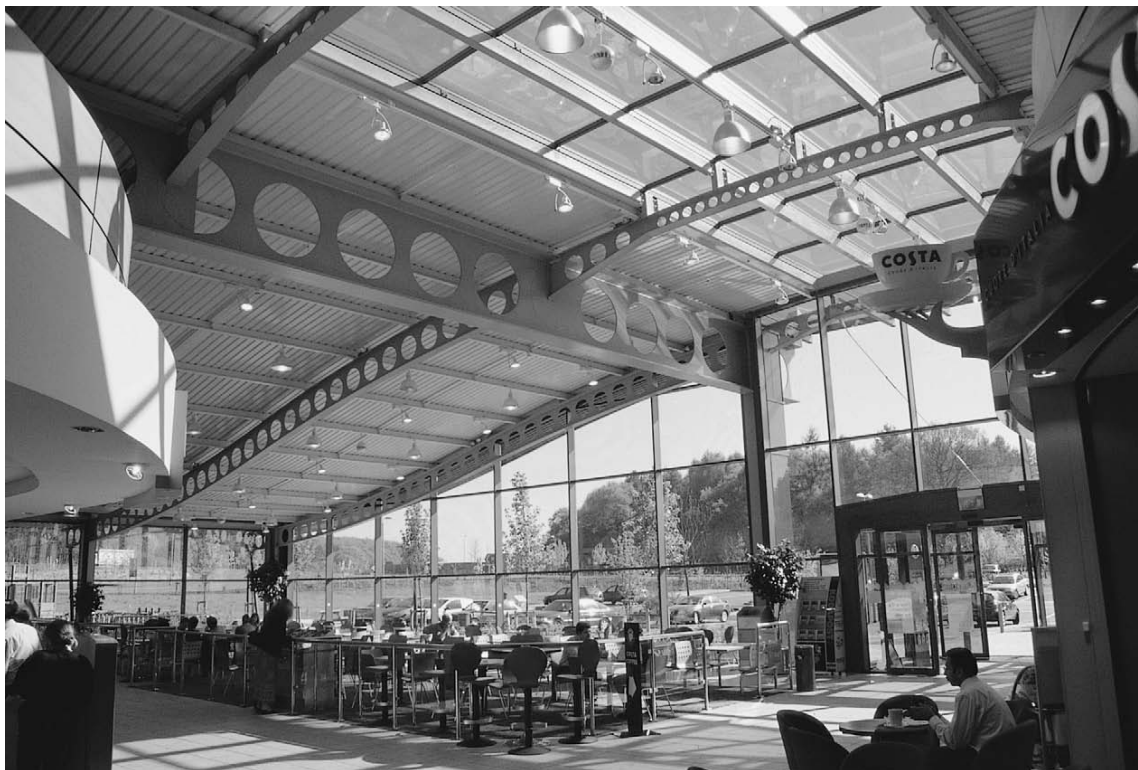
4.2 Curved cellular beam used for architectural effect
