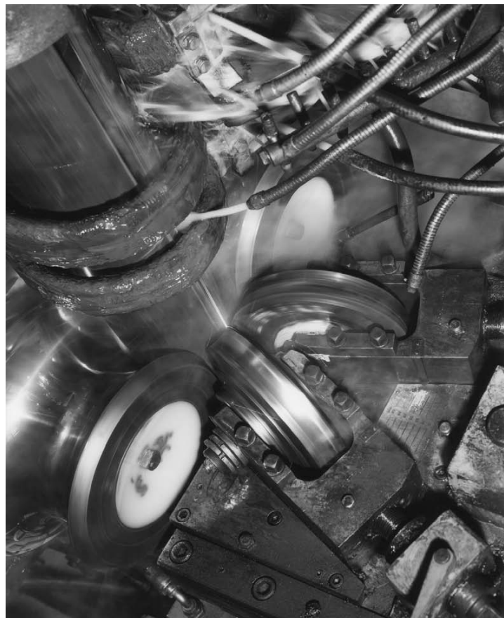
11.1 Strip being formed and welded into a tube
