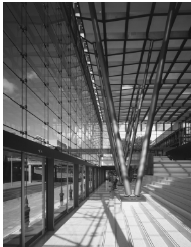
9.10 Tension structure to support glazing at the University of Bremen, Germany (architect: Jan Stormer)
