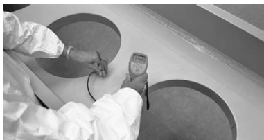
13.3 Intumescent coating to cellular beam being measured for its coating thickness
