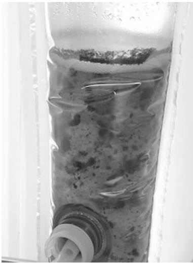
Fig. 4.2 Scale-up cell suspension culture of sweet basil ( Ocimum basilicum L.) in a 5-l airlift bioreactor (Osmotek Lifereactor)
