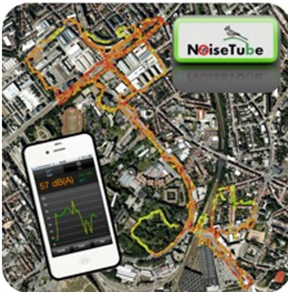
Fig. 5 NoiseTube: noise pollution monitoring using mobile phones (courtesy of Vrije Universiteit Brussel BrusSense group, http://www.brussense.be/ )
