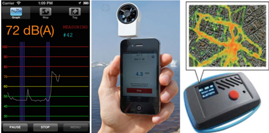
Fig. 1 Smartphone app to measure noise pollution (NoiseTube), wind sensor for smartphone, wearable air pollution sensor (Sensaris)
