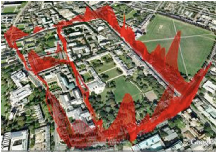
Fig. 3 Real-time pollution monitoring using hand-held sensors carried by pedestrians (courtesy of Cambridge Mobile Urban Sensing, http://www.escience.cam.ac.uk/mobiledata/ )
