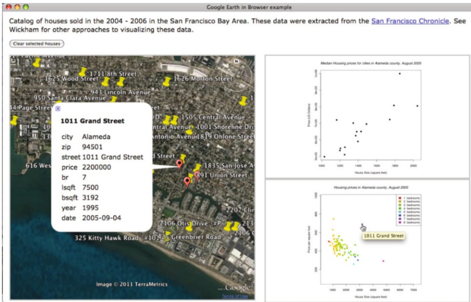
Figure 17.11: Web Page of San Francisco Housing Prices, Linking Google Earth and SVG Scatter Plots. This screenshot displays an HTML page with Google Earth embedded in it. To the right of Google Earth are two scatter plots, which are Scalable Vector Graphics (SVG) documents embedded in the HTML page. The SVG documents, Google Earth plug-in, and JavaScript in the HTML page enable the viewer to dynamically interact in several ways with these displays of housing sales. As shown heret, when the mouse hovers over a point, the address appears in a tool tip, and when we click on this point, a paddle is added to Google Earth to make it easier to see it. Additionally, when we click on this paddle, further information about the house pops up. A click on the button above the plug-in will remove all of these additional paddles from the display so only the yellow pushpins remain.
