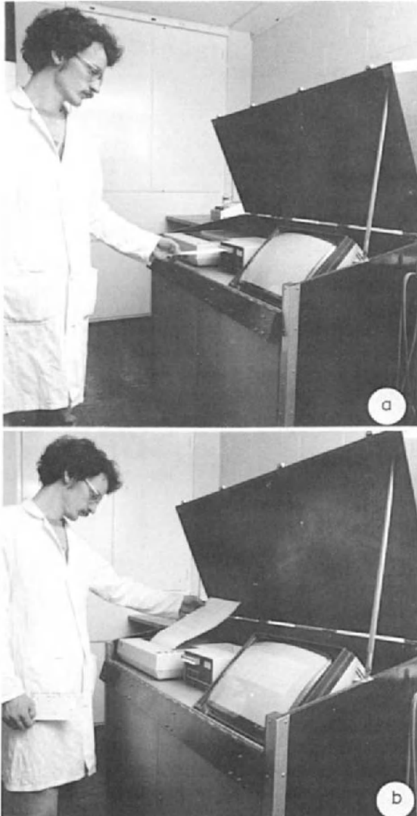
Figure 4.6.(a) The computer-marked MCQ system. The hardware is housed in a portable cabinet. The computer, the discs and the paper are housed inside the cabinet and the doors are kept shut during the test. The students have access to the monitor, optical mark-sense card reader and printer in the upper compartment. (b) The MCQ system in use for student self-assessment. (c) Part of a typical output sheet. (d) Part of a card on which the students record their responses.
