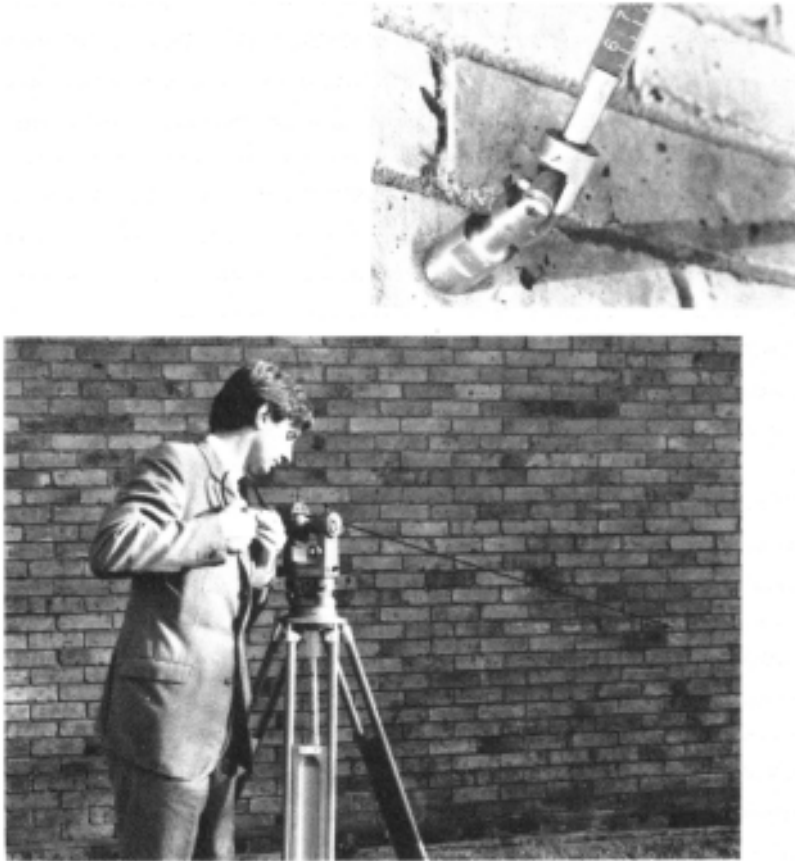
Figure 2.3 Taping to a BRE levelling station.
