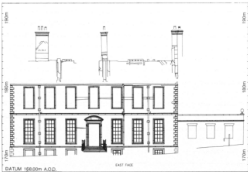
Figure 3.3 Uppark House, east elevation. This drawing was produced by AMC Ltd using a Galileo Siscam Digicart 40 photogrammetric instrument. All final plots on the Uppark project were computer generated using AutoCAD. (Reproduced with the permission of the National Trust; Architects, The Conservation Practice.)
