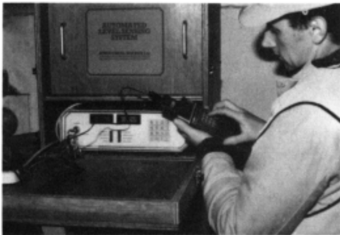
Figure 5.4 Down-loading data from an automated level sensing system.
