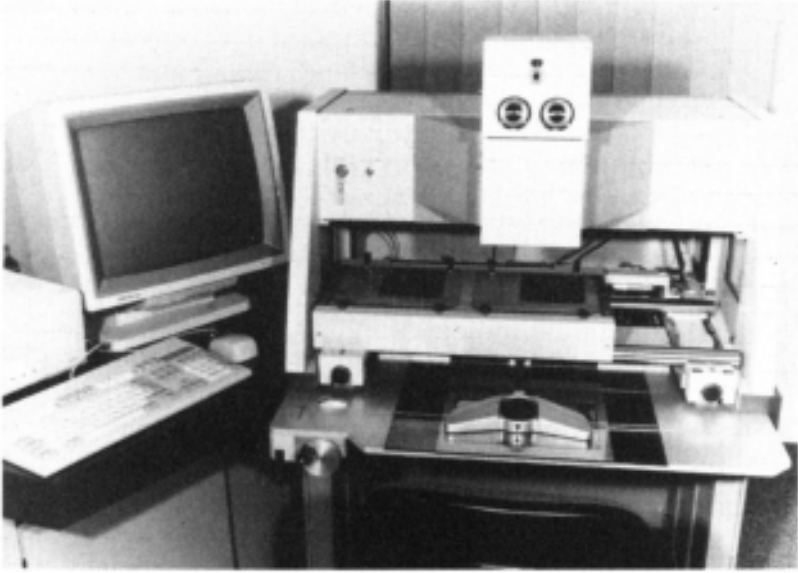
Figure 3.13 Galileo Siscam Digicart 40. This analytical instrument is driven by a '386 PC' and relies on a high-resolution graphics screen to portray the recorded data rather than the conventional plotting table. (Photograph courtesy of AMC Ltd.)
