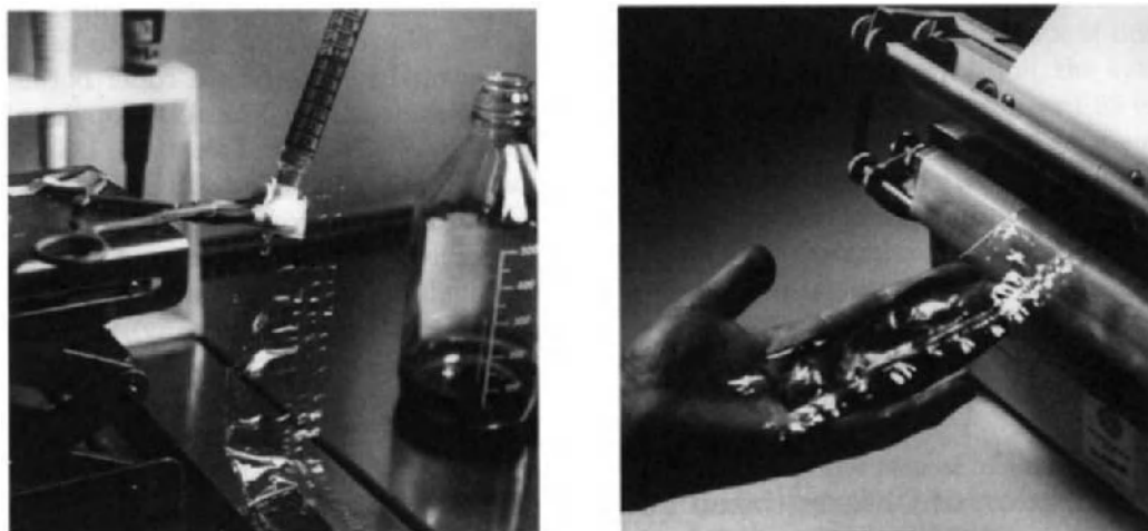
Figure 3. Teflon bags for long-term culture of MOs. (A) A bag is attached to a stand with self-adhesive tape and filled with cell suspension. (B) The bag is closed with a sealing device before incubation.
