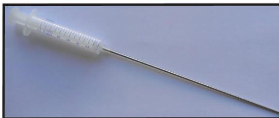
Figure 7.15 Homemade syringe for inserting cement pastes at the bottom of NMR tubes.
