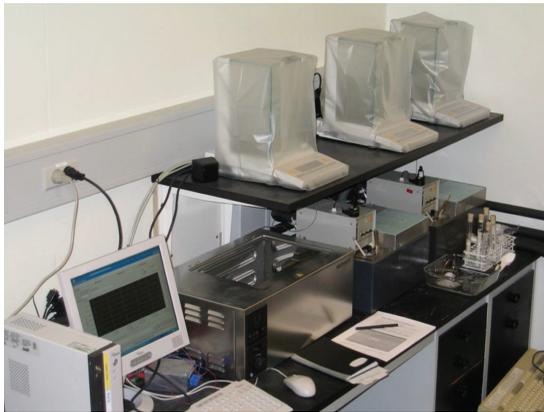
Figure 3.8 Setup for automatic measurement of chemical shrinkage using gravimetry.
