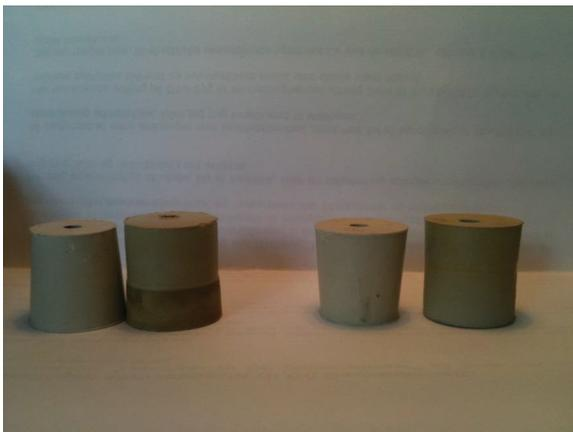
Figure 3.14 Stoppers before and after exposure to oil for several months.
