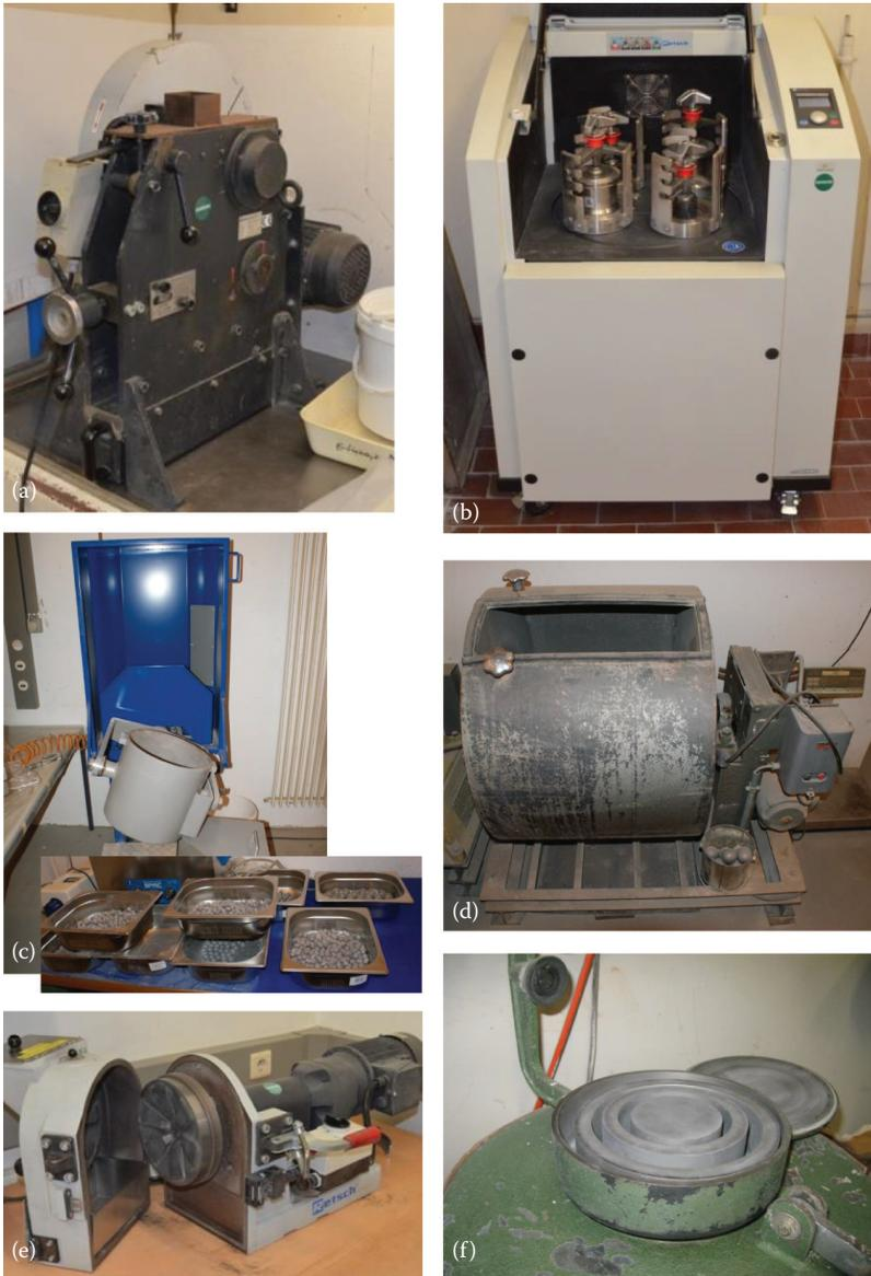
Figure 1.4 Examples of crushers and laboratory mills used for particle size reduction of raw materials for cementitious binders: (a) jaw crusher; (b) planetary ball mill; (c, d) laboratory ball mills; and (e, f) disk mills. (Courtesy of R. Snellings, Flemish Institute of Technological Research, Mol, Belgium [a, b, e], and J. Rossen, École Polytechnique Fédérale de Lausanne, Switzerland [c, d].)
