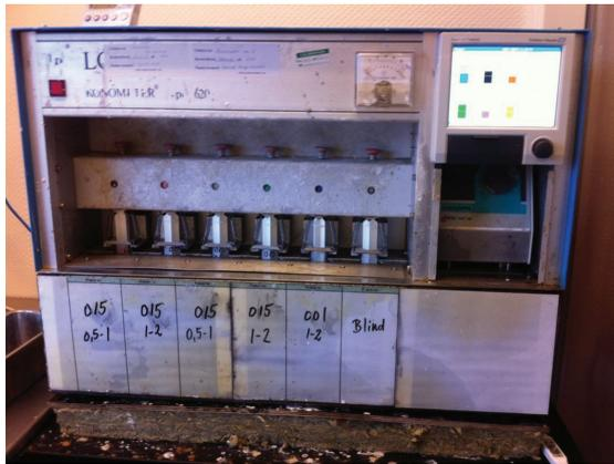
Figure 3.9 (Well-used) Konometer for automatic measurement of chemical shrinkage. Here it is used for testing the alkali reactivity of sand. (Courtesy of Søren Lolk.)
