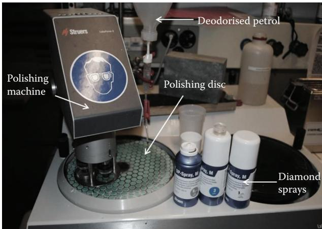
Figure 8.14 Polishing machine with the polishing disc and the diamond sprays.
