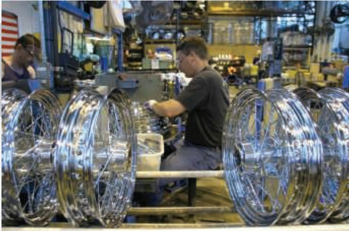
Wheel assembly modules are prepared in a work cell for JIT delivery to the assembly line.
