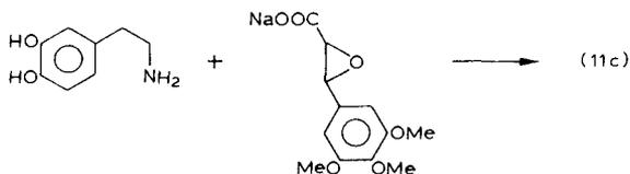
*Scheme 2.1.* Use of glycidate precursor in Pictet-Spengler synthesis of trimetoquinol, pH 2.3 for 115 h.
