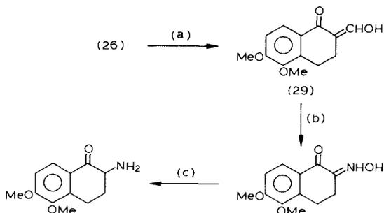
Scheme 2.9. Reagents (a)  $\text{HCOOEt}$ ,  $\text{NaOMe}$  (b)  $\text{NANO}_2$  (c)  $\text{H}_2$ ,  $\text{Pd-C}$ .
