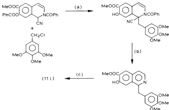
Scheme 2.4 The Reissert route to 1-substituted isoquinolines. Reagents (a) NaH-DMF (b) NaOMe then HCl (c)  $H_2PtO_2$  then  $LiAlH_4$ .
