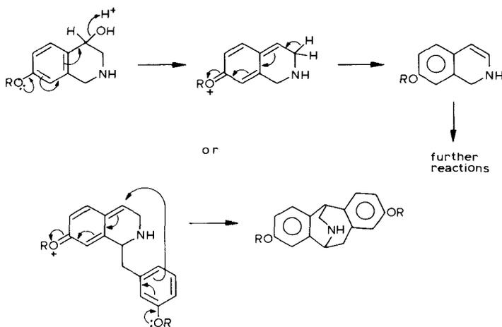
Scheme 2.5. Instability of 7-oxygenated 4-hydroxy-1,2,3,4-tetrahydroisoquinolines in acid
