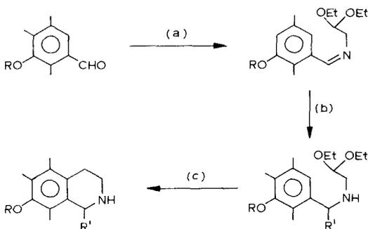
*Scheme 2.2.* Bobbitt synthesis of tetrahydroisoquinolines. Reagents (a)  $\text{H}_2\text{N.CH}_2\text{.CH(OEt)}_2$ , (b)  $\text{H}_2$  and catalyst or Grignard (c) 6N HCl,  $\text{H}_2$ , Pd on C.
