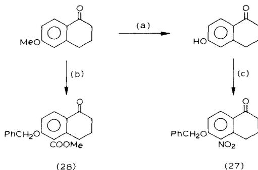
Scheme 2.8. Reagents (a) conc HBr or  $AlCl_3$ , (b) 8 steps (c) nitration, separation of isomers, benzylation.
