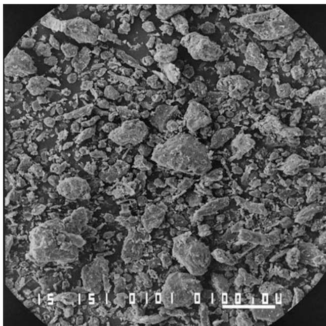
Fig. 4.3 Particle size variation in the manually (in a mortar with a pestle) crushed Nifedipine tablet (Adalat® 10 mg retard). Scale bar in SEM is 100 \mu\text{m} [29]
