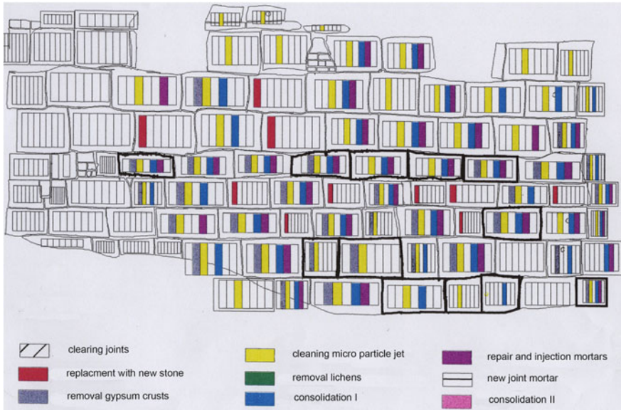
Fig. 7.23 Nuremberg Maxtormauer. Mapping of complex conservation projects with the help of simplified indication of measures (Wendler 1997)
