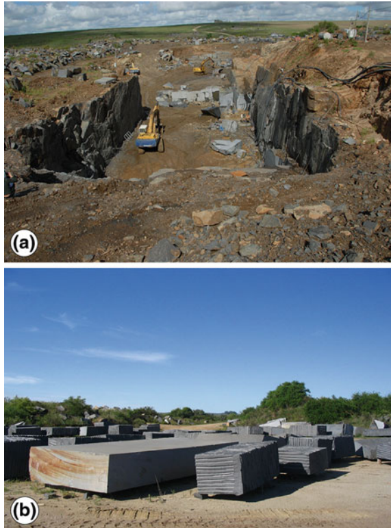
Fig. 2.36 a Quarry of black dolerite in Uruguay and b Blocks of Negro Absoluto and Oriental
