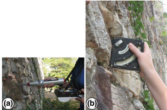
Fig. 6.23 a Digi-Schmid and b Duroscope being used in the field
