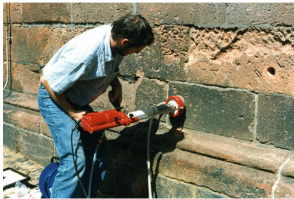
Fig. 6.39 Sampling of drill cores ( d = 5 cm) on weathered parts of a facade
