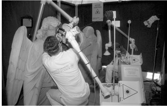
Fig. 7.34 Nd:YAG Laser with articulated arm in practical employment (Figure by Bauer-Bornemann)
