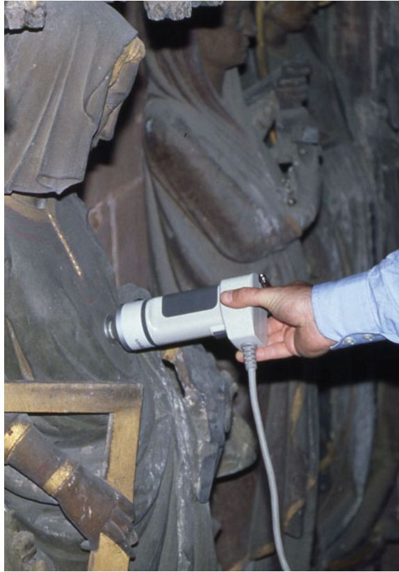
Fig. 6.38 Color measurements with chromameter at the Freiburg Minster, Germany
