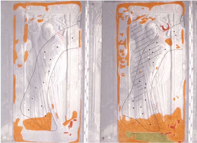
Fig. 6.17 Gravestone from Eberbach Monastery (Germany) with minimal map ( left ) and maximal map ( right ) of damages recorded by different workers. After Eickelberg et al. (1990), for explanation see text (Figure by the Zollern-Institut, Deutsches Bergbaumuseum)
