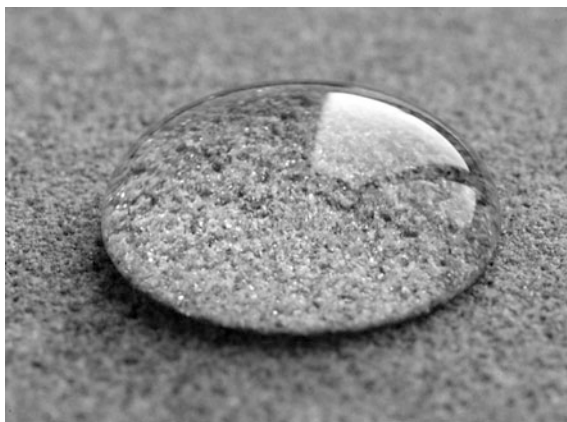
Fig. 7.70 Water droplet on a water repellent stone surface (Figure by Leisen)
