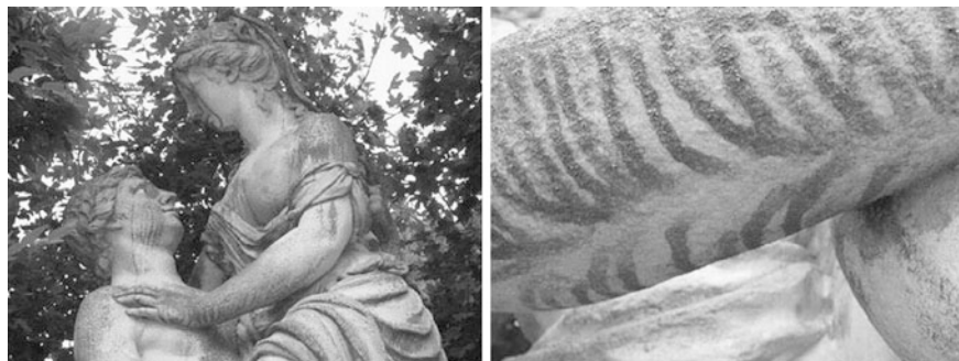
Fig. 7.86 Cyanobacterial and fungal growth on water runnels caused by water repellent (Sterzinger Marble, Schönbrunn, Vienna, Austria) (Figure by Sterflinger)
