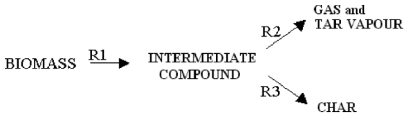
Fig. 11.1. Model of pyrolysis mechanism with intermediate compound
