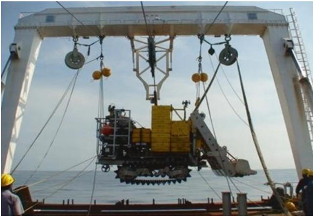
**Fig. 10.37** Launching of underwater mining machine
