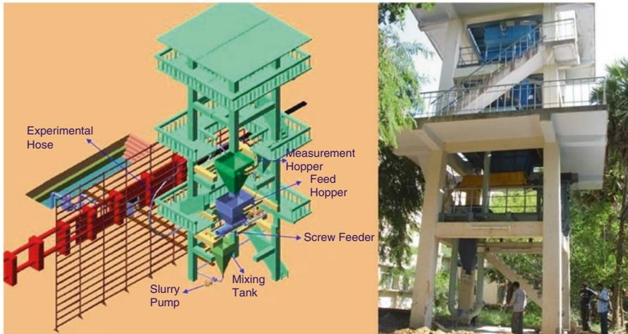
Fig. 10.12 Experimental setup for study of manganese nodule flow through hoses
