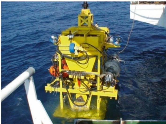
Fig. 10.25 Artificial nodule laying system being launched
