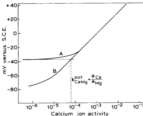
*Figure 2.1.* The effect of constant magnesium ion concentration on the response of the PVC electrode to varying calcium ion activities: A,  $5 \times 10^{-3} \text{ mol dm}^{-3} \text{ Mg}^{2+}$ ; B,  $\text{Ca}^{2+}$  only
