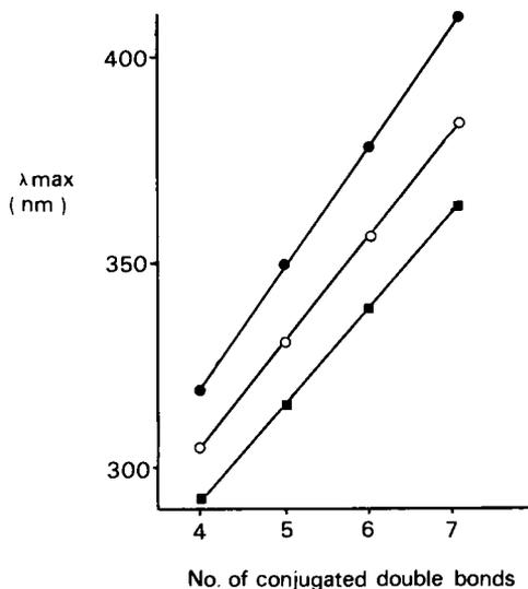
*Figure 3.1. Relationship between UV absorption maxima and the number of conjugated bonds in the polyene chromophore. The wavelength of the three major absorption peaks are shown*
