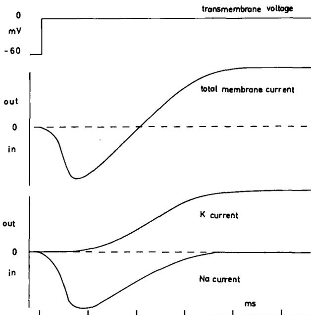
Figure 1.8. Hypothetical diagram illustrating the time course of events in a voltage-clamped excitable membrane. At time zero the membrane potential is changed stepwise from  $-60$  mV to zero, and is held there. In consequence ionic currents flow across the membrane, the net current is first inward, but then reverses to give a maintained outward current. The contributions of sodium and potassium currents which account for the total membrane current are shown
