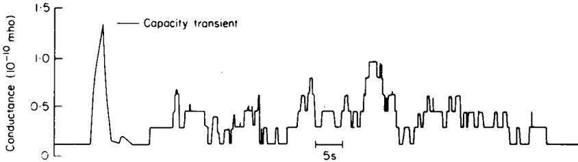
Figure 1.2. Gramicidin conductance transitions with time in a bilayer membrane made from glyceryl mono-oleate and *n*-hexadecane. The aqueous phases were 0.5 M NaCl, the transmembrane potential was 100 mV, temperature 23°C [207]
