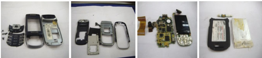
Description: Dissembled mobile phone (mobile phone case, electronic circuit, battery). Photo by: Witthawin Sangprasert
