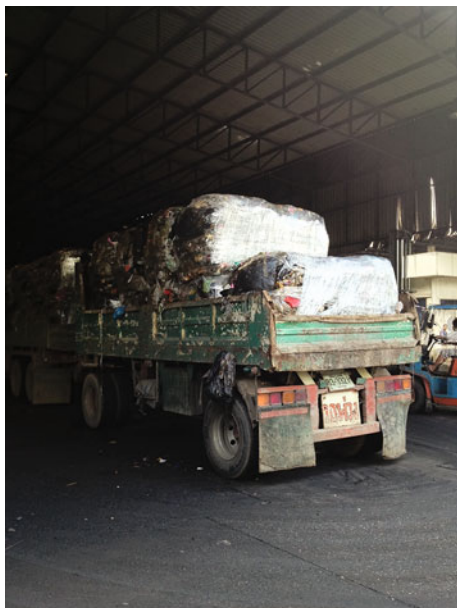
Description: Municipal wastes are wrapped with plastic at transfer station before transporting to landfill. Photo: Chanathip Pharino
