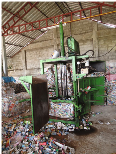
Description: Wastes compression machine to reduce volume easing transportation. Photo by: Amornchai Challcharoenwattana
