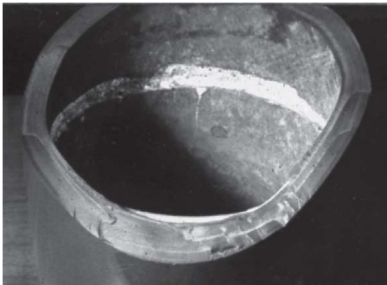
Figure 6.8 ESC failure of a 250 mm diameter PVC water main (the white deposit is excess cement)
