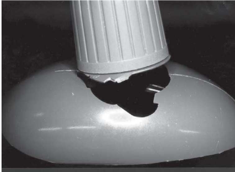
Figure 6.32 ESC failure of a PVC bottle
