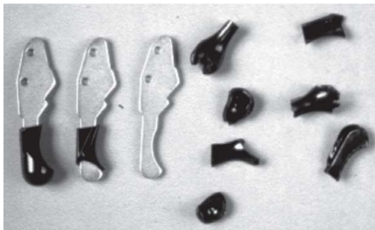
Figure 5.16 Disintegrated outsert mouldings
