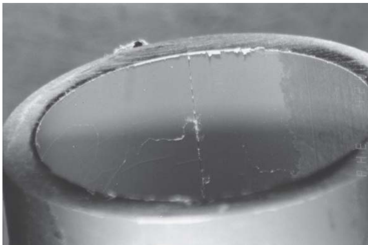
Figure 6.37 An axial crack in an ABS pipe
