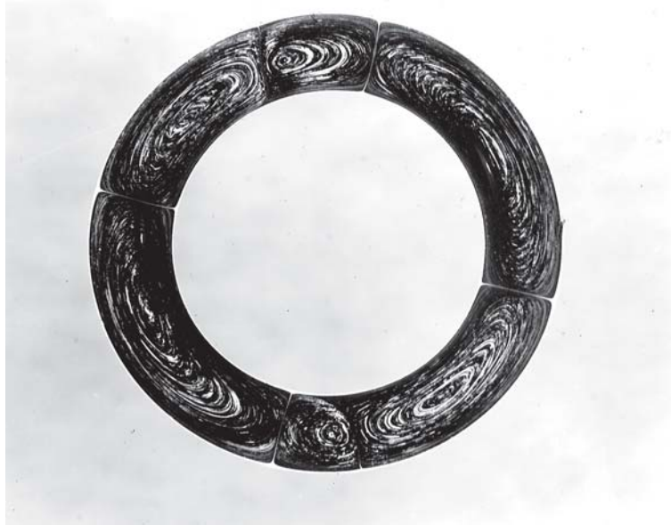
Figure 3.12 A microtomed cross-section reveals poor carbon black distribution
