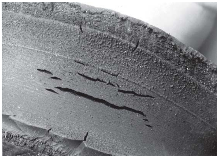
Figure 2.14 Cracking/splitting of the bore caused by bending
