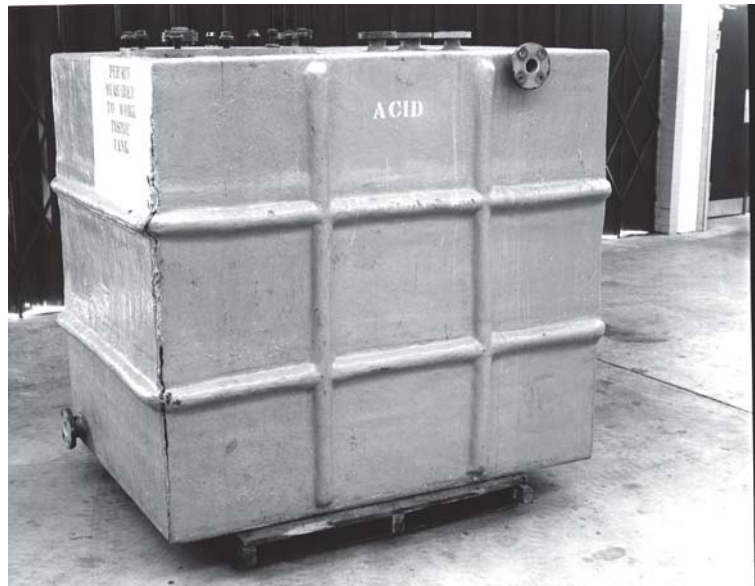
Figure 5.17 The failed GRP tank
