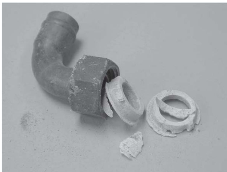
Figure 5.14 The failed acetal fitting
