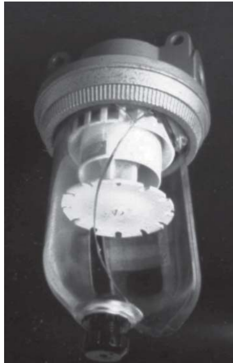
Figure 1.5 Failed polycarbonate filter bowl
