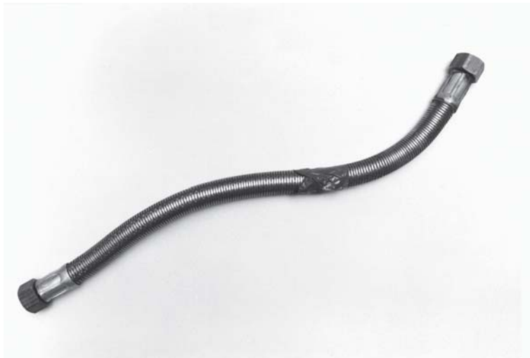
Figure 2.13 The failed hose
