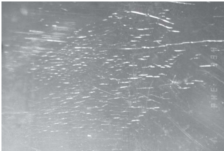
Figure 6.38 Crazing on the outside surface of a polycarbonate filter bowl
