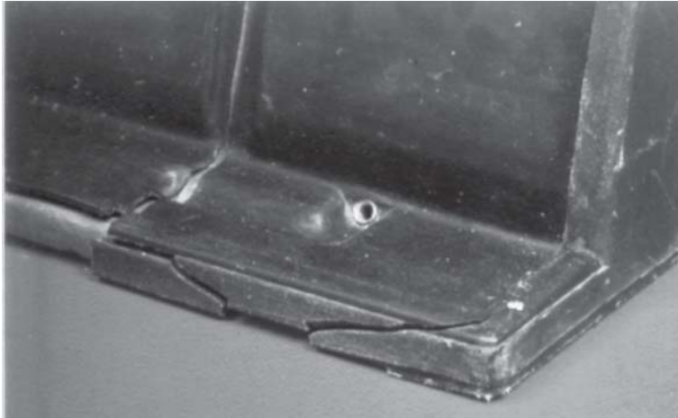
Figure 6.34 Cracked wine cooler
