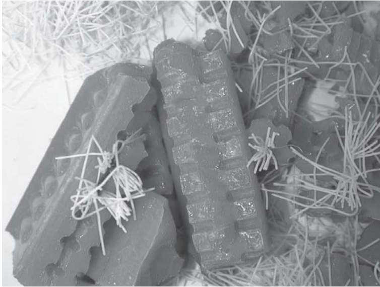
Figure 6.31 Disintegrated scrubbing brush
