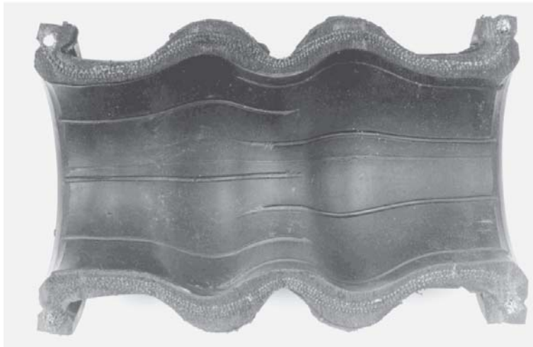
Figure 2.9 Bellows cross section (unused)
