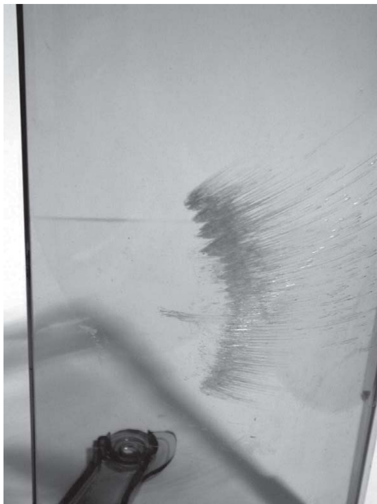
Figure 5.2 Splay marks on a polycarbonate moulding due to inadequate drying
