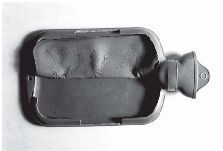
Figure 2.18 The inner surface of the failed side reveals degradation
