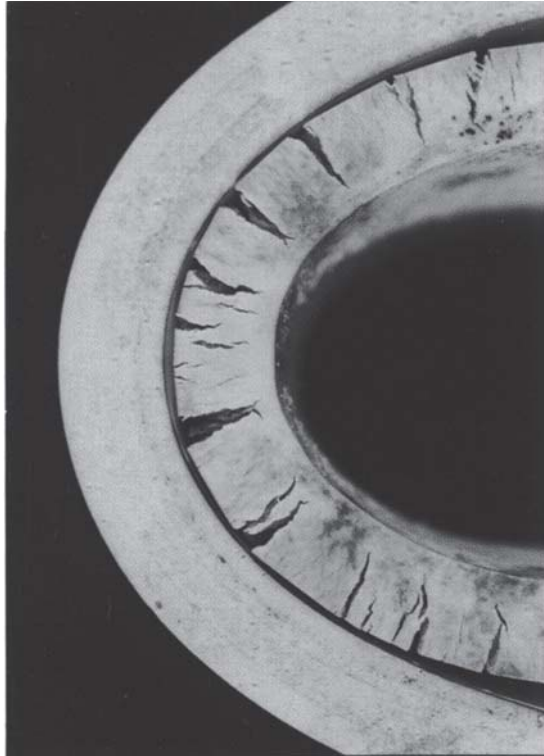
Figure 7.4 Polyurethane shoe soles after 90 days of soil burial under stress, with and without a biocide
