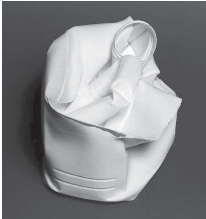
Figure 6.19 Buckled PE container
