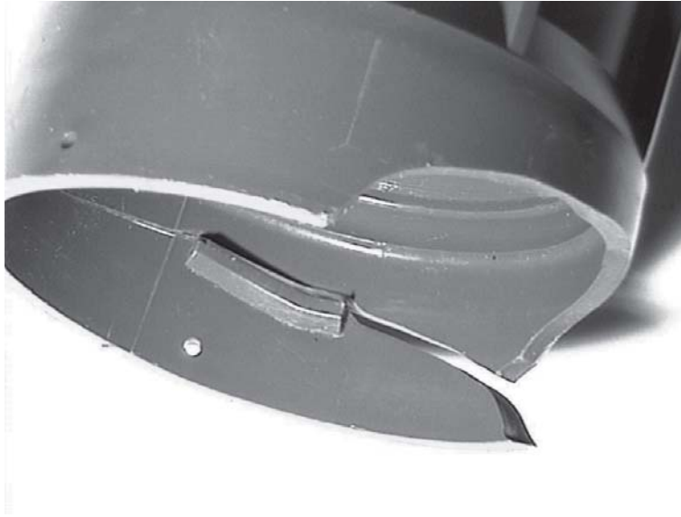
Figure 6.14 Typical example of a failed cap. Initiation is at the lug
