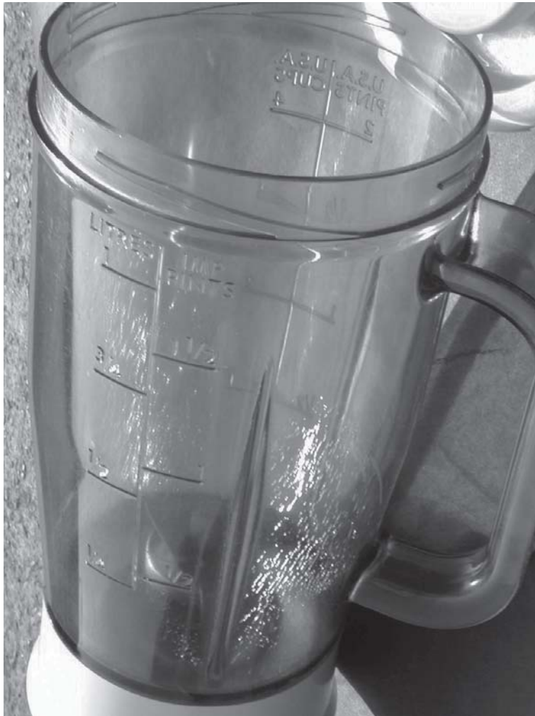
Figure 6.35 Extensive crazing on the internal surface of a polycarbonate mixing jug
