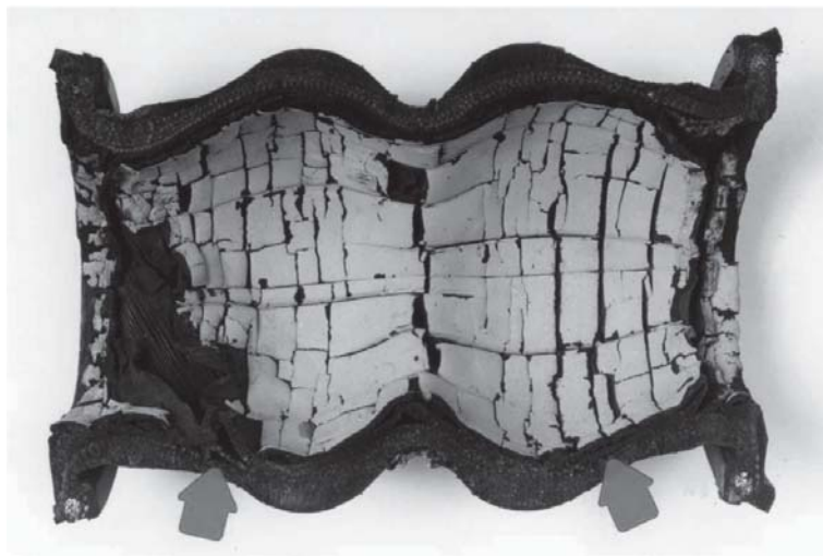
Figure 2.10 Cross section of a failed bellows
