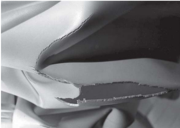
Figure 6.20 Close-up showing classical linear stepped microcracking due to ESC
