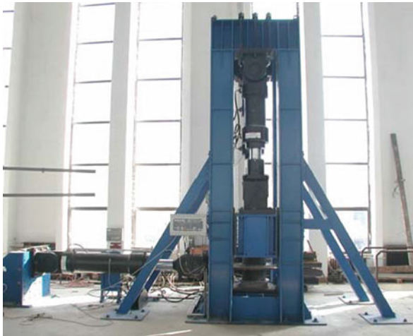
Fig. 17.16 Big two-componental testing machine
