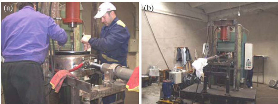
Fig. 17.15 Production of prototype large bearing: (a) assemblage of the shim plates and rubber sheets in the mold (b) curing process
