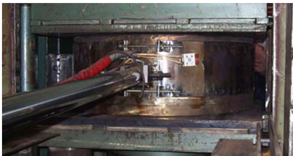
Fig. 17.22 Vulcanization of large isolators
