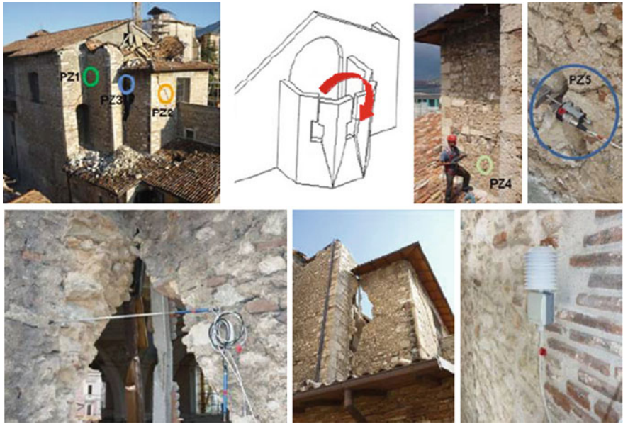
Fig. 20.12 View of the apsidal area of St. Mark church: displacement and temperature-relative humidity sensors positioning
