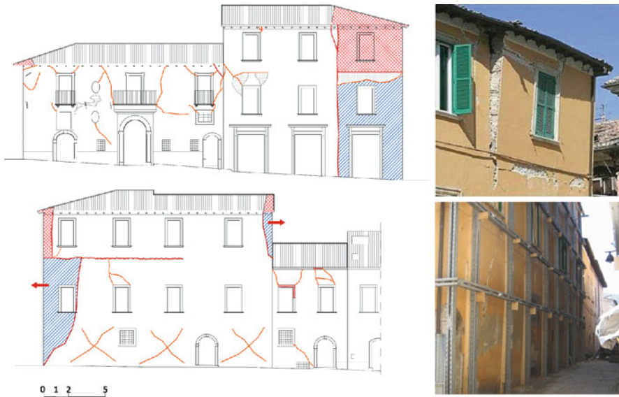
Fig. 20.26 Damage state in the building in Piazza della Prefettura: elevations and pictures
