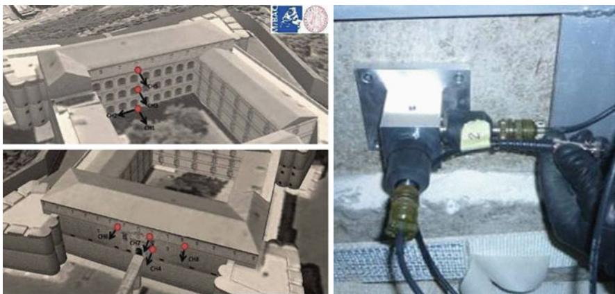
Fig. 20.18 L'Aquila castle: left – localization of the acceleration transducers; right – base acceleration transducers (CH1, 2) and acquisition unit
