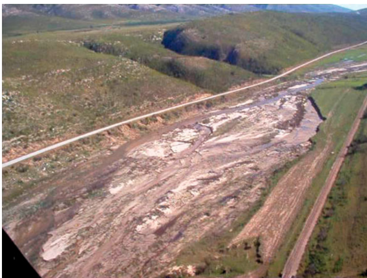
Fig. 16.8 An aerial photograph taken from a helicopter of the main floodplain of the Kromme River after a large flood event. The floodplain was once covered by large palmiet wetlands, specially adapted withstand the force of the flood waters. The removal of the palmiet wetlands has destabilized the system, causing massive headcuts which lower the water table and reduce the agricultural potential of the land
