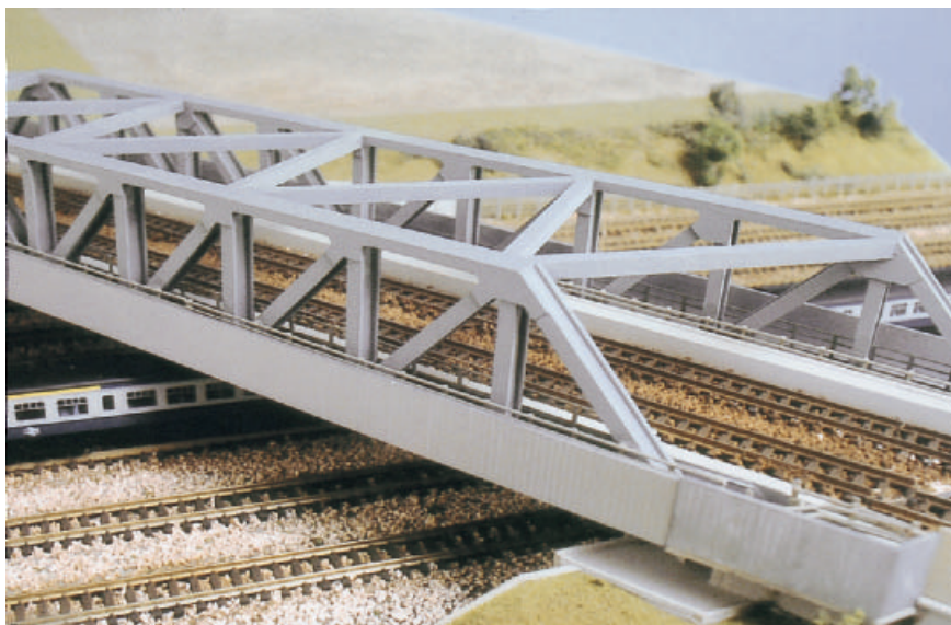
Fig. 7.4. Model of welded truss railway bridge.
