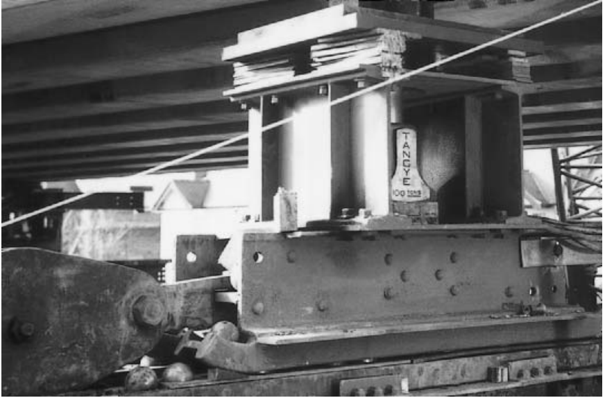
Fig. 7.9. 100 tonne rolling-in trolley.
