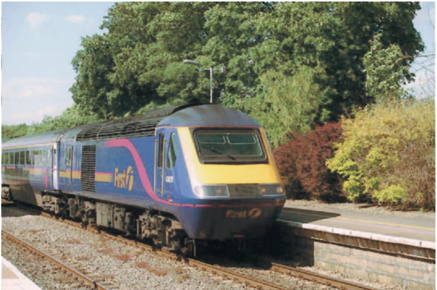
Fig. 3.8. Diesel-electric locomotive (photo by Paul Walker).
