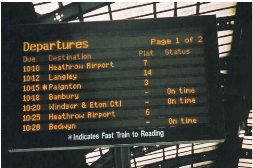
Fig. 11.3. Dot matrix departure indicator.
