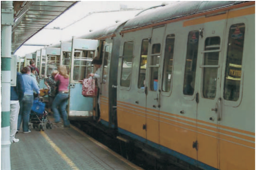
Fig. 3.6. Old DC electric multiple unit stock with 'slam' doors (photo by Paul Walker).
