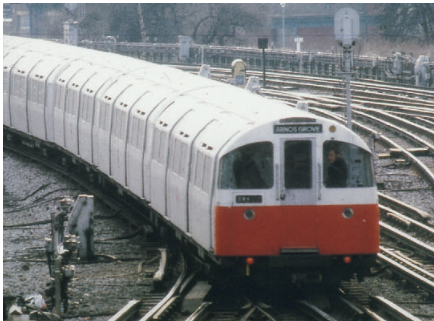
Fig. 3.5. Electric multiple unit underground train.
