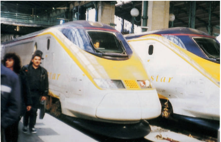
Fig. 3.7. Channel tunnel ‘Eurostar’ electric stock which can run on either AC or DC.
