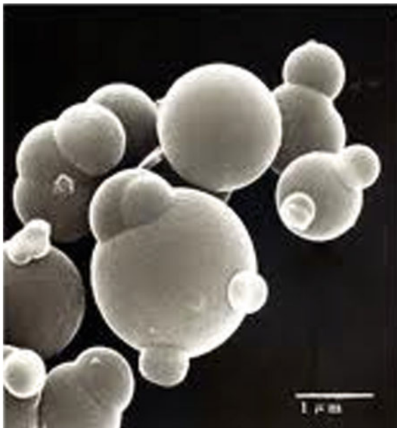
Figure 8. SEM image of marigranules.
