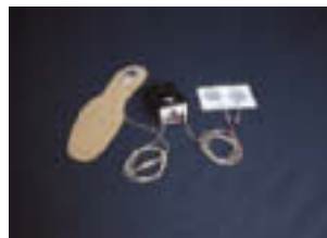
Figure 14.3 Left: the Odstock Dropped Foot Stimulator. Right: patient with incomplete spinal cord injury using the dropped foot stimulator.
