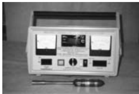
Figure 13.5 Seager Model 14 electroejaculator with rectal probe. By courtesy of Professor SWJ Seager, Washington DC, USA.
