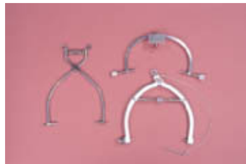
Figure 5.2 Cone (left), Gardner-Wells (upper right), and University of Virginia (lower right) calipers.
