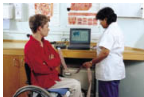
Figure 12.2 Force sensing array: pressure mapping can be used to assess pressure distribution, which helps to prevent skin breakdown.
