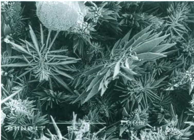
Figure 1a. Spectacular bladed crystals formed from 10 000 ppm copper solution.
