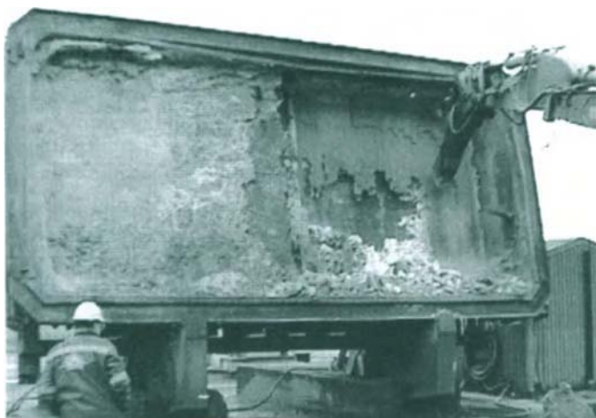
Figure 1. The dismantling of the cathode. The right half was crushed down and homogenised and should be representative for the “total cell”. The left half was separated into three different cuts as visualised in Figure 2.
