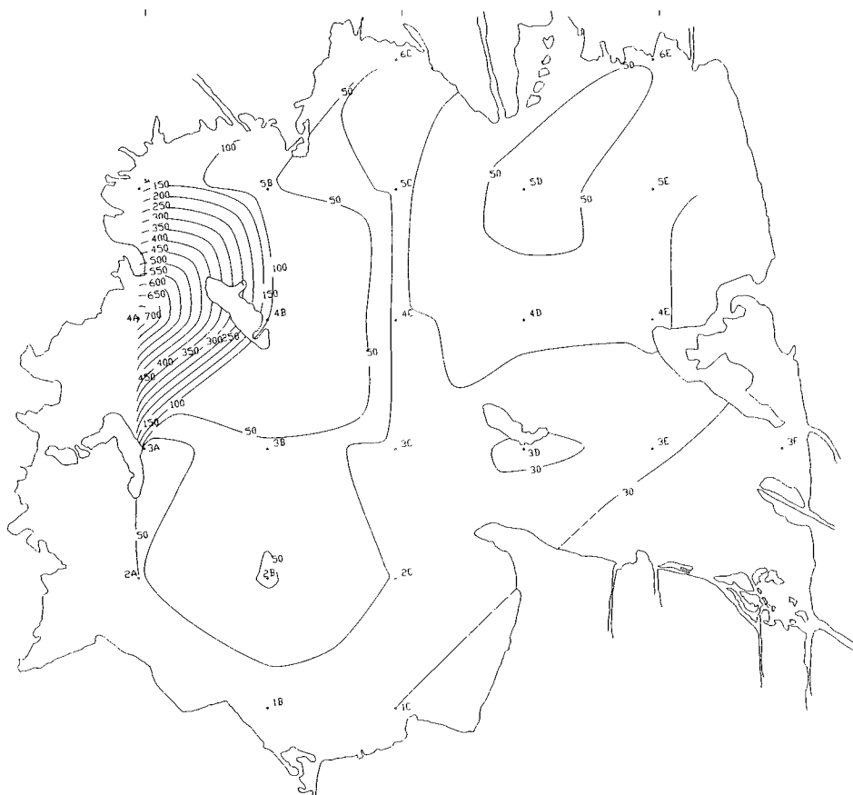
Fig. 2 Iso-Concentration lines in ppm of Chromium. Sample-point 4A more than 700 ppm Chromium
