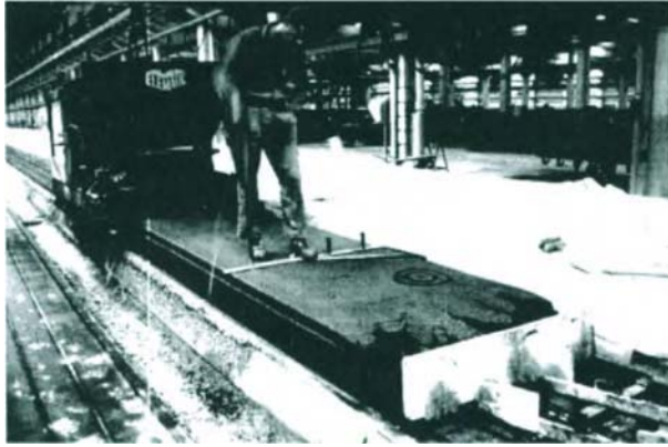
Figure 1. End line waste of hollow core slab units
