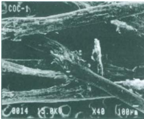
Figure 1. Coir fiber surface morphology
