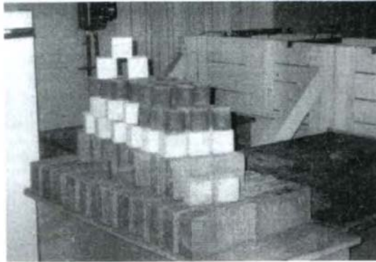
Figure 5. Test specimens of fine cementless ash - slag concrete
