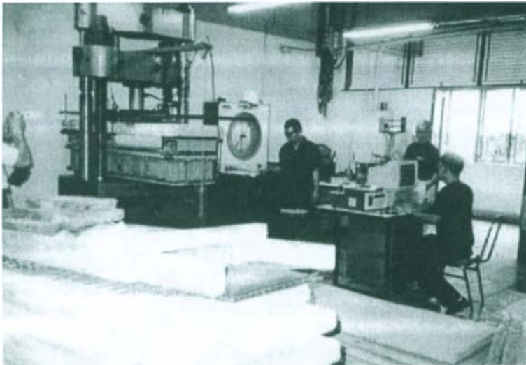
Figure 3 Flexural test setup of the ribbed panel
