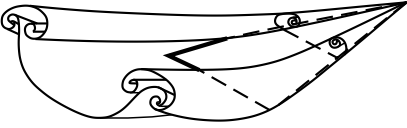
Fig. 6.56. Steady vortex separation at the leading edge of a delta wing
