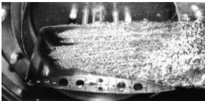
cloud cavitation, Re = 10^7, \sigma = 1.2
