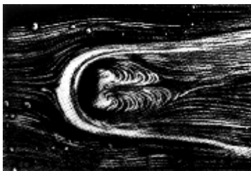
Fig. 4.75. Paint visualization and structure of a wall flow perturbed by a vertical plate (horseshoe vortex) A. Hinderks
