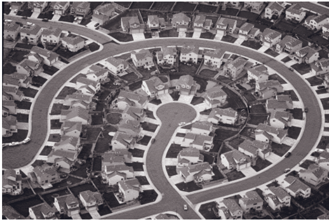
Figure 34.6 Suburban planning designed for car transport. Very few intersections or cross-connections between streets means that a pedestrian has to walk long distances between places that are relatively close.
