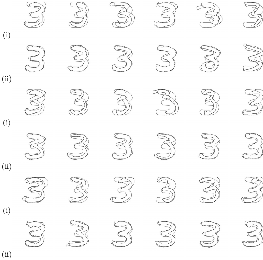
Fig. 3. Global registration using the affine transformation model. (i) Initial pose, (ii) affine-invariant registration (the same target contour is used).
