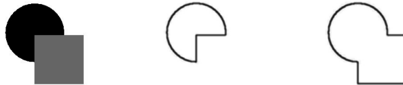
Fig. 1. Level lines and T-junction. Depending on the gray-level configuration between shapes and background, level lines may or may not follow the objects' boundary. In any case, junctions appear where two level lines separate. Here, there are two kinds of level lines: the occluded circle and the shape composed of the union of the circle and the square. The square itself may be retrieved by difference.
