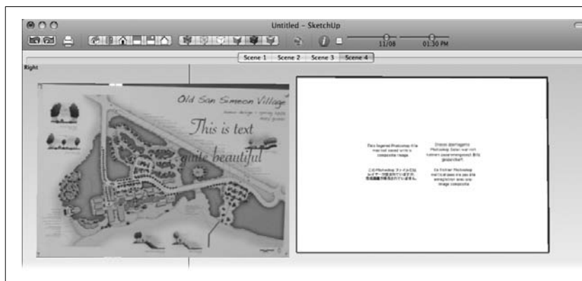
Figure 13-7: An identical image was saved with (left) and without (right) Photoshop’s compatibility option. The image saved without the compatibility option displays an error message when you try to import it.
