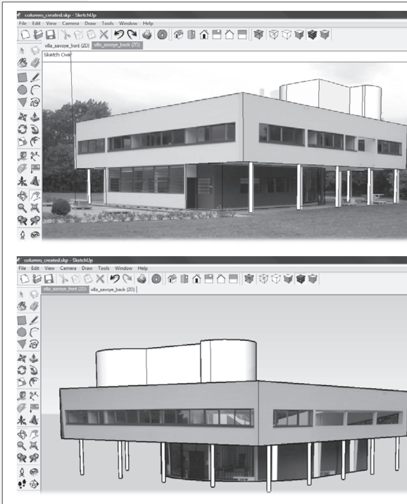
Figure 10-25: This view of the front of Villa Savoye has photo textures applied to some of the surfaces.
