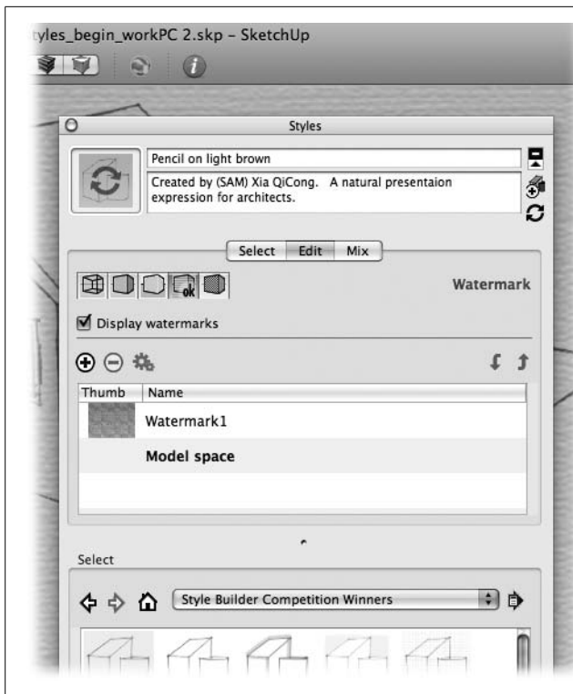
Figure 6-34: The “Pencil on light brown” style uses a watermark that simulates a textured paper, and the edge setting gives the look of a pencil drawing.
