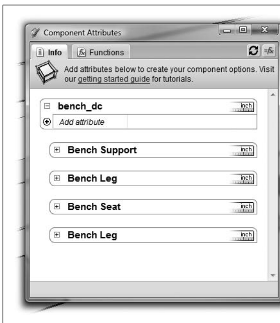
Figure 14-9: Two windows are related to dynamic components. The Component Attributes window, shown here, is used to create dynamic components. You must have SketchUp Pro to access this window. The Component Options window (page 334) lets anyone using SketchUp work with dynamic components.
