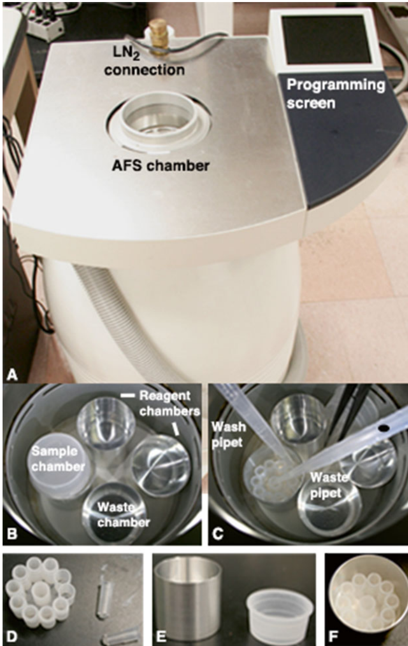
Fig. 5 Freeze substitution device and materials. (a) Leica AFS2. Note the LN 2 connection for filling the machine using a funnel attachment, the AFS chamber where samples will incubate, and the mouse-controlled programming screen. (b) Close-up of AFS chamber containing universal chambers. A minimum of one waste chamber and one reagent chamber should be present along with any sample-containing universal chambers. (c) Wash setup in AFS chamber. One pipet is used for washing with new solution and the other marked waste pipet is used for disposing of waste to prevent contamination. (d) Flow-through ring and mesh-bottom vial inserts. Cut a notch in one of these rings to aid in recording sample position. Insert a mesh-bottom vial tube into each sample-containing arm of the ring. (e) Universal chamber and plastic lid (f) Universal chamber containing flow-through ring with mesh-bottom vial inserts. Samples will incubate in this chamber, while reagents and waste are stored in empty universal chambers. Cover this chamber with the inverted plastic lid when not in use to prevent evaporation of solutions
