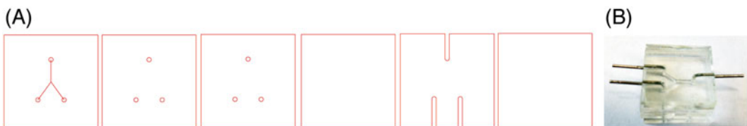
Fig. 1 A Y-Junction for microfluidics made of 1/32" clear cast acrylic. (a) The design of the six layers of the part. (b) An image of the part
