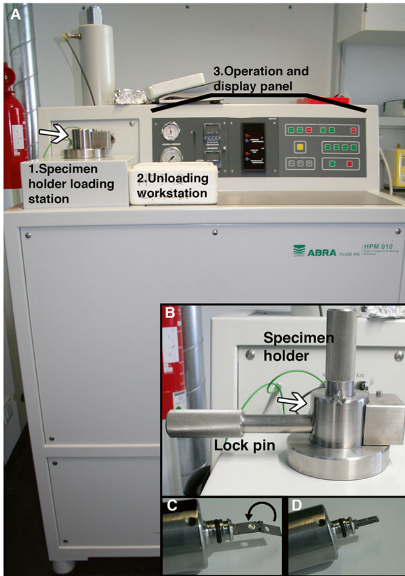
Fig. 1 (a) BAL-TEC HPM010 high-pressure freezer machine. (b) Specimen holder loading station with inserted specimen holder and lock pin. Hold the specimen holder with the right hand and the lock pin with the left hand to minimize the transfer time of the frozen sample in the specimen holder to the unloading workstation. (c) Open specimen holder containing specimen carrier. Close hinge and rotate to tighten as seen in (d) before loading into the loading station
