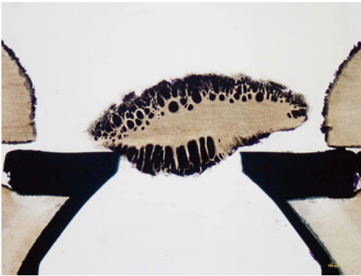
Fig. 8.11 Thin section with crystal violet staining of a used Provox 2 voice prosthesis. The valve flap shows infiltrating biofilm deposits over nearly the whole flap surface. The deformation of the flap form can cause insufficient valve closure
