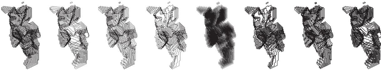
*top left:* EZCT Architecture & Design Research with Hatem Hamda and Marc Schoenauer, studies on optimisation: computational chair design using genetic algorithms, 2004. The 'Bolivar' model is evaluated for a multiple load strategy (it is always stable, whatever way the seat is positioned). This model (prototype and drawings) is part of the Centre Pompidou Architecture Collection. © Philippe Morel (original drawings © Centre Pompidou).
