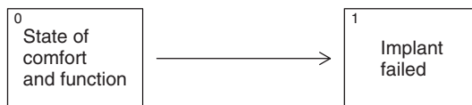
Figure 15.2 Two-state survival model for implant failure. The failure probabilities are described by the transition intensity between state 0 and 1.
