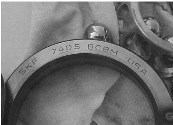
Figure 6.10 Failed CRD outboard bearing.
