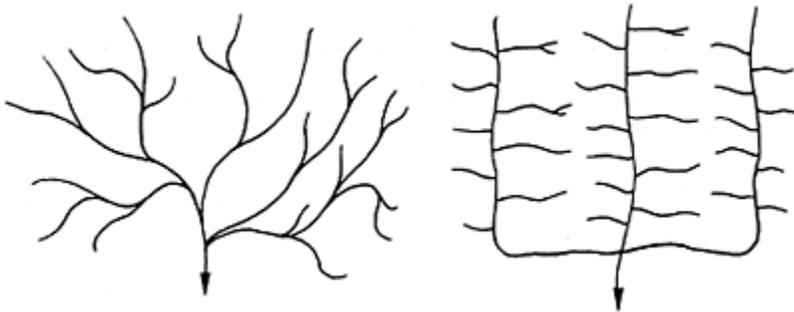
**Figure 12.1** Dendritic and trellis drainage pattern.
