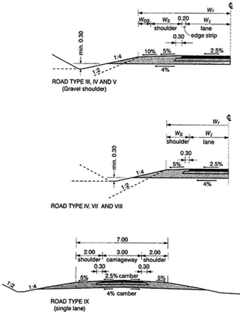
Figure 9.2 Typical cross-section (ref. 3).
