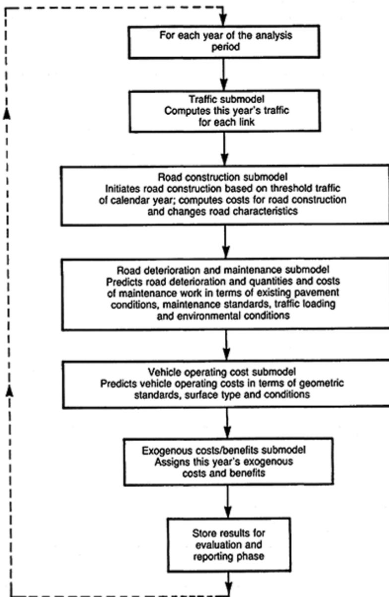
Figure 4.1 Simulation of a link alternative (ref. 4).
