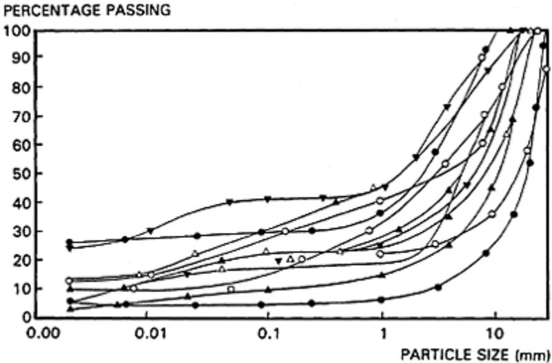
**Figure 13.2** Typical gradings of lateritic gravels (ref. 2). (Crown copyright; reproduced with the permission of the Controller of HMSO.)
