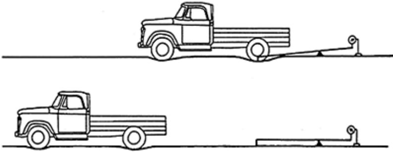
Figure 16.8 Benkelman beam measurement.
