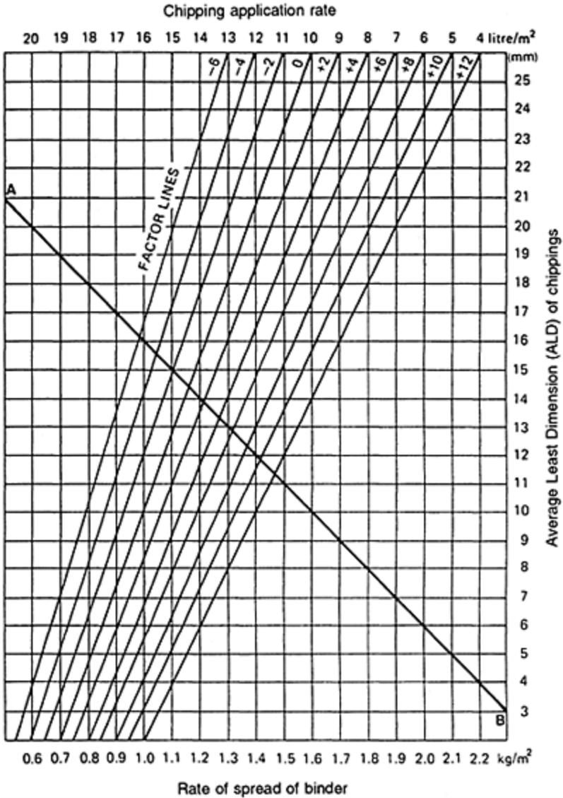
**Rate of spread of binder.** The rate of spread of cutback bitumen is determined by the intercept between the factor line and the appropriate ALD line. For penetration bitumen the rate determined from the chart should be reduced by 10%. For emulsified bit the percentage of bitumen in the emulsion. For slow traffic or steep climbing the rate should be reduced by 10%. For fast traffic or steep down grades the rate should be increased by 10 to 20%.
