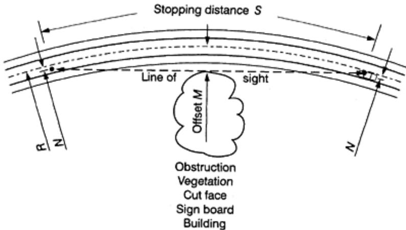
**Figure 8.1** Minimum offset to obstruction adjacent to curve.
