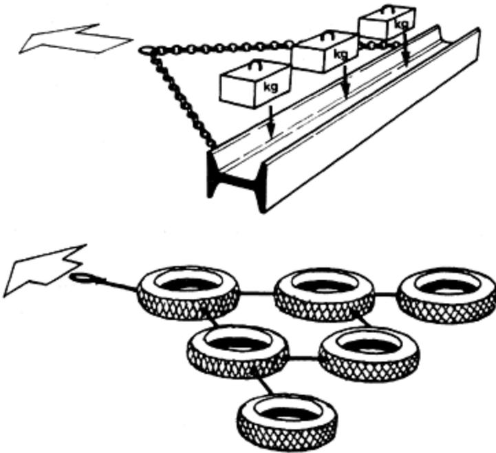
**Figure 20.6** Beam drag and tyre drag (ref. 2).
