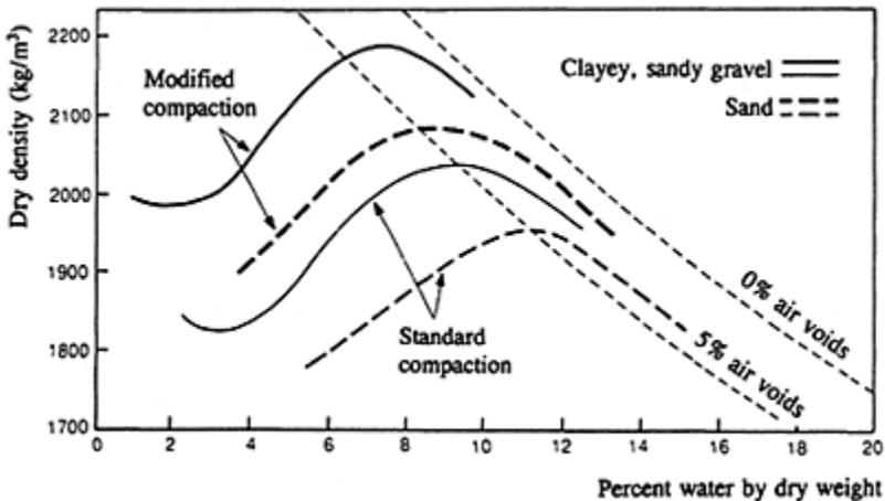
**Figure 12.10** Example of compaction curves (ref. 7). (Crown copyright; reproduced with the permission of the Controller of HMSO.)
