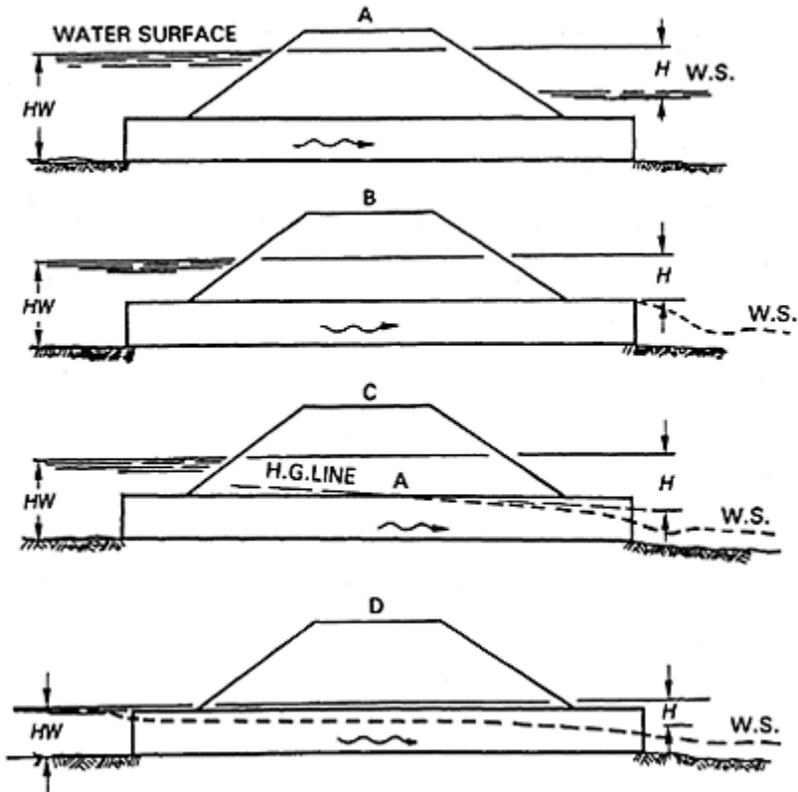
Figure 11.7 Outlet control (Transportation Research Board, ref. 3).
