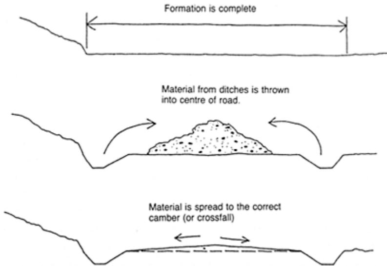
**Surface** drainage prevents water from damaging the road by leading it off the road quickly. This is done by shaping the road so that the water can flow freely into the side drains.
