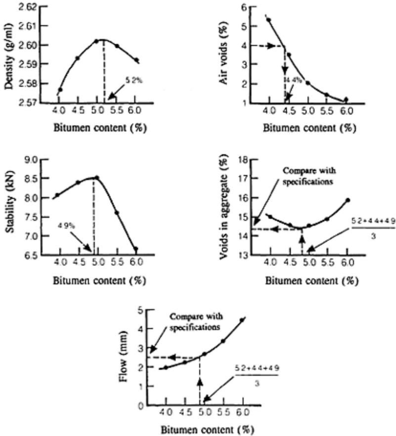
Figure 15.8 Results from a Marshall test (ref. 4).
