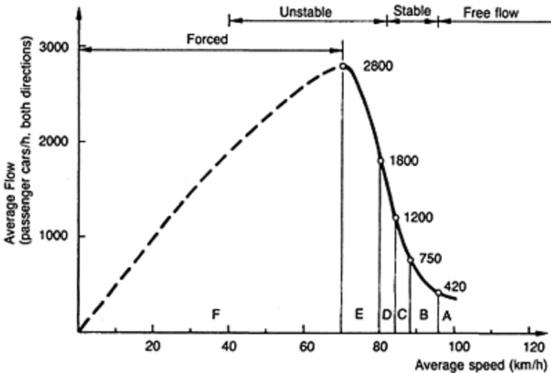
Figure 7.1 Speed-flow diagram.
