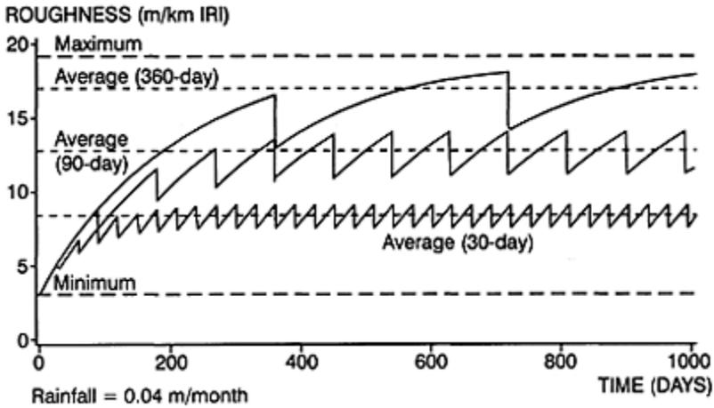
Figure 4.5 Roughness progression and effect of grading (ref. 6).
