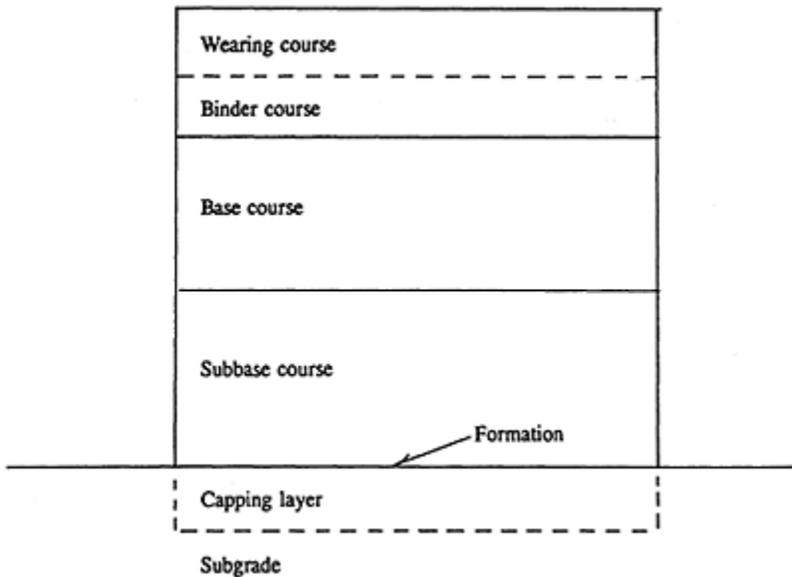
**Figure 14.7** Terms used for the different pavement layers.
