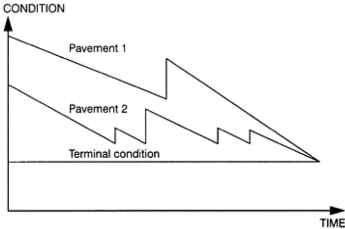
**Figure 16.1** Deterioration as function of time.
