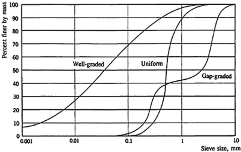
**Figure 12.7** Particle size distribution curves.
