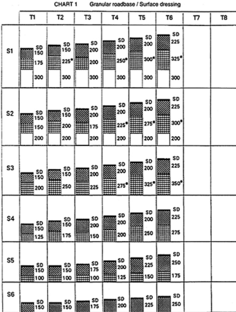
Note: 1 \* Up to 100mm of sub-base may be substituted with selected fill provided the sub-base is not reduced to less than the roadbase thickness or 200 mm whichever is the greater. The substitution ratio of sub-base to selected fill is 25mm:32mm.
