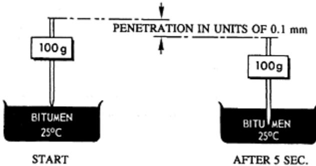
**Figure 15.1** Penetration test.
