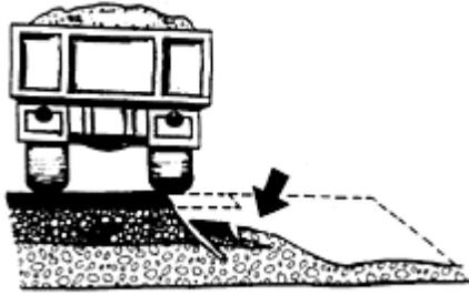
**Figure 20.4** Broken edges (ref. 2).
