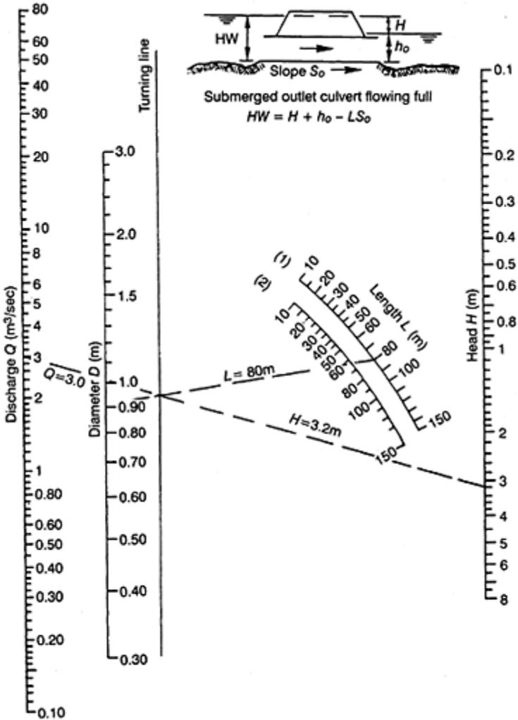
Scale (1): Inlet with groove end (socket end) projecting, and inlet with groove end (socket end) and headwall.
