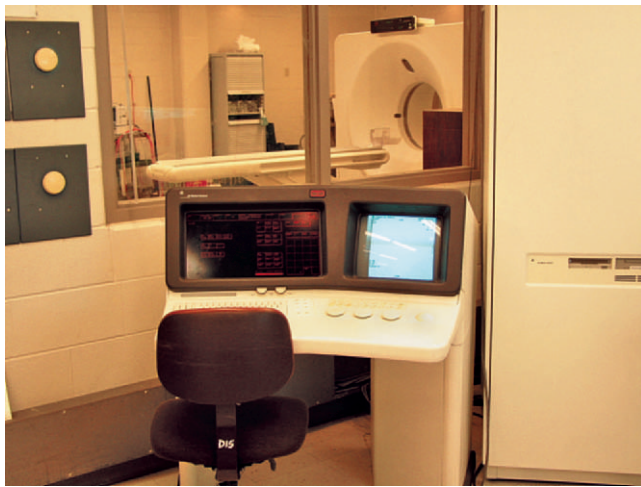
FIGURE 10-37 Typical layout of a computed tomography imaging suite, with the workstation in the foreground, shielded from the x-ray tube, gantry, and moveable patient couch in the adjacent room.
