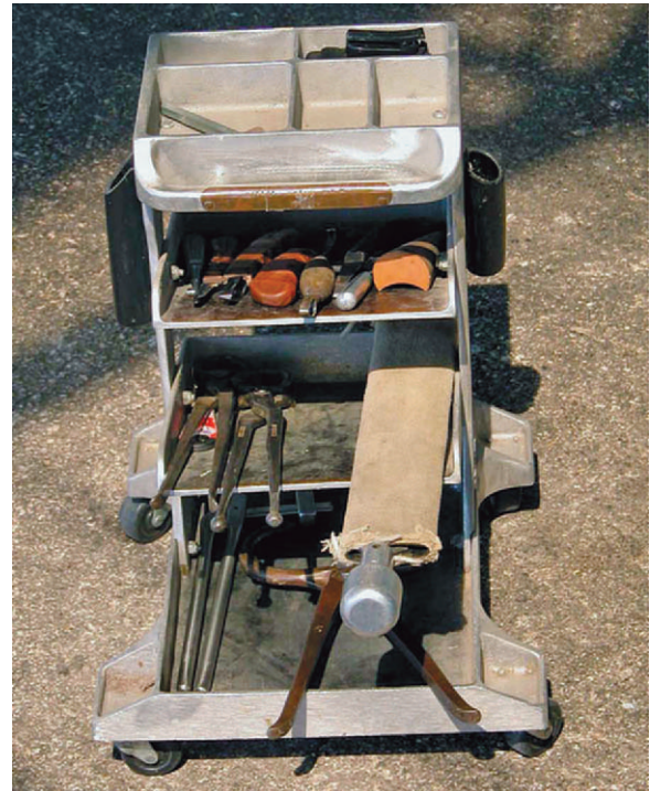
FIGURE 8-1 A rolling set-up for farrier equipment is useful in a hospital setting. The wheels allow the user to quickly move the equipment away from the horse in the event of a problem.
