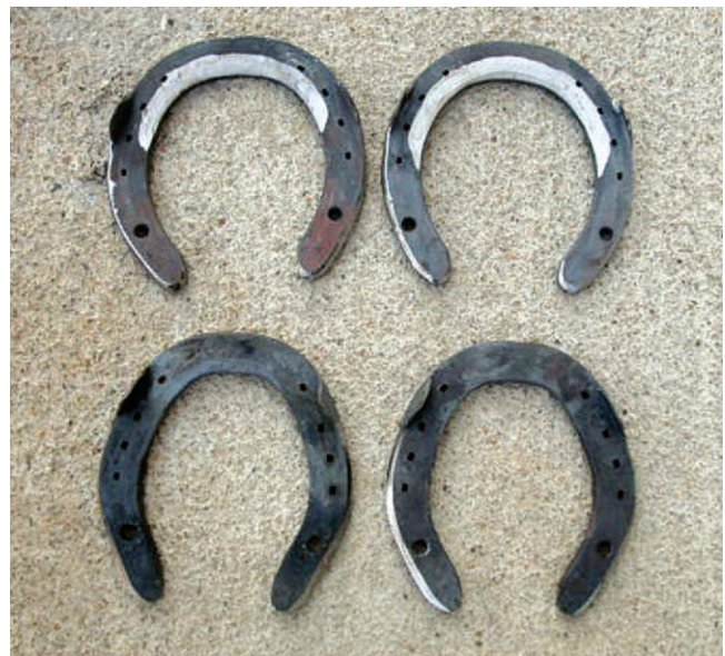
FIGURE 22-20 Foot surface of set of spare shoes demonstrating light concaving and heavier than usual boxing.
