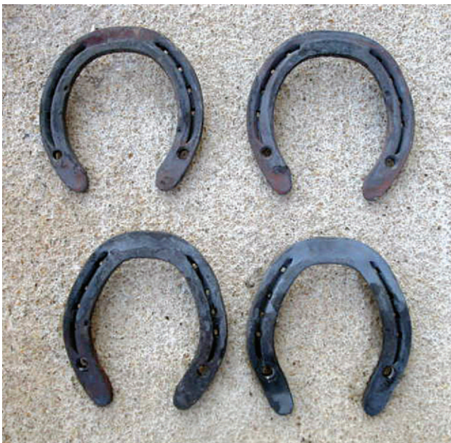
FIGURE 22-14 Ground surface of spare shoes showing marks on the outside indicating right or left and stud holes. The spare shoes should be as precisely fit as if they were going to be nailed on the horse.
