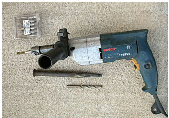
FIGURE 22-15 Implements for drilling and tapping shoes: \frac{3}{8} -inch \times 16-tpi taps, power tapper, stud punch, and \frac{5}{16} -inch or P-sized drill bit.
