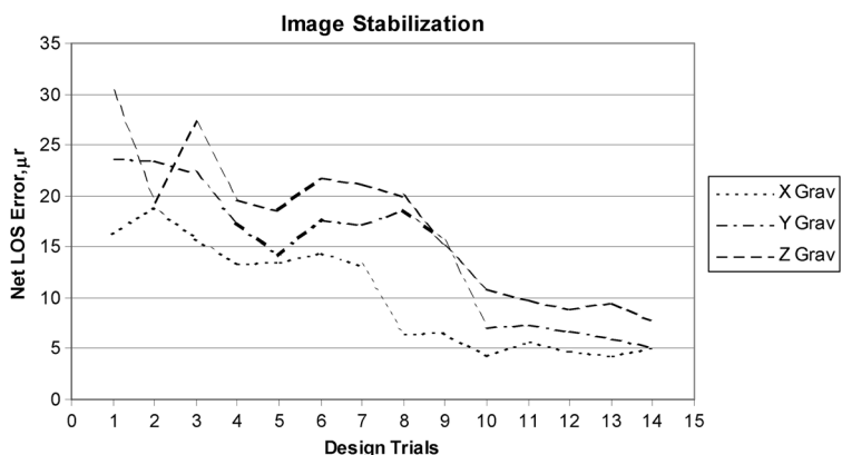
Figure 7.20 The history of reducing the LOS errors in Patran/Nastran (reprinted from Ref. 10).
